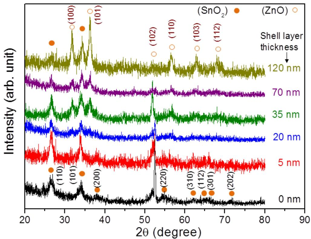
**Fig. S2** XRD patterns of SnO<sub>2</sub>-ZnO CSNs prepared with different numbers of ALD cycles. For comparison, an XRD pattern of bare SnO<sub>2</sub> nanofibers is included.
