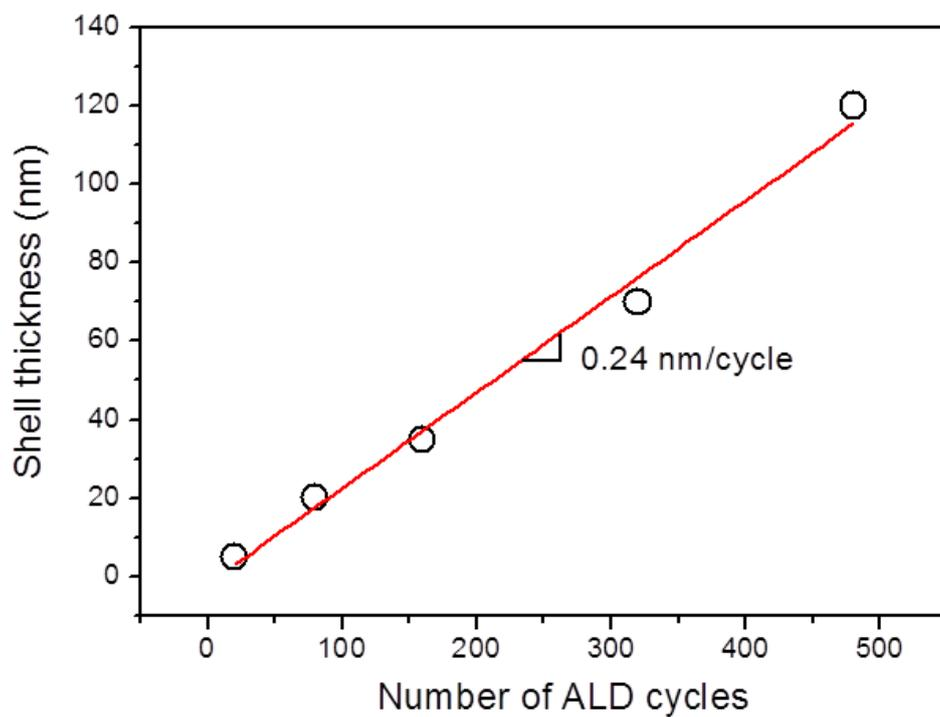
**Fig. S1** ZnO shell thickness of SnO<sub>2</sub>-ZnO CSNs as a function of the number of ALD cycles. The slope corresponds to the growth rate of ZnO shells.
