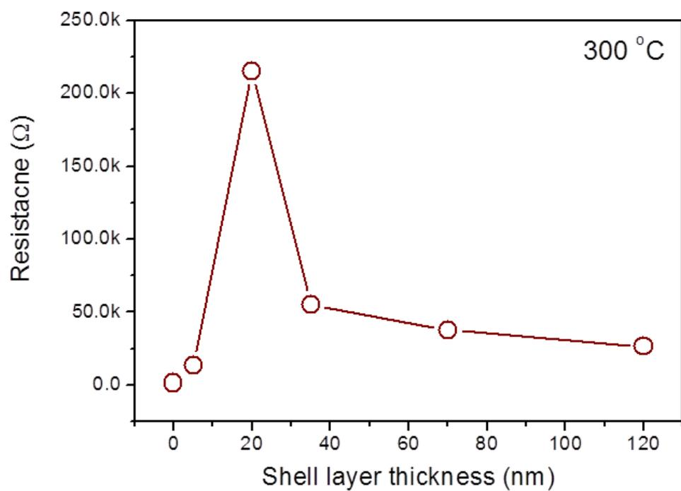
**Fig. S3** Change of the resistance of SnO<sub>2</sub>-ZnO CSNs as a function of shell thickness in air at 300 °C.
