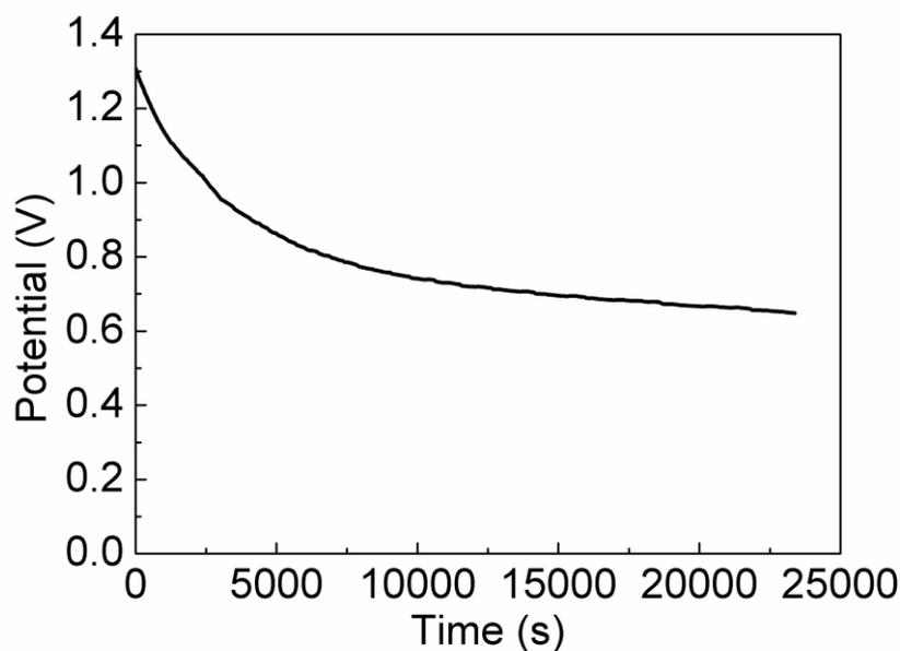
**Fig. S14** Self-discharge curve of our supercapacitor device obtained immediately after charging to 1.3V. The result shows that our supercapacitor self-discharges from 1.3V to 0.65 V in a long time of 6.5 h indicating the low self-discharge property.
