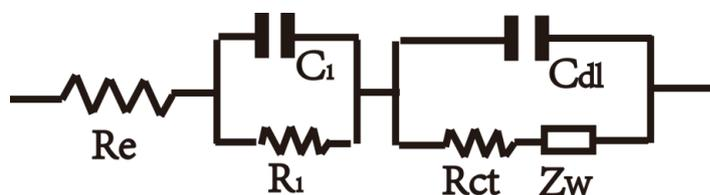
**Fig. S9** The electrical equivalent circuit used for fitting impedance spectra.
