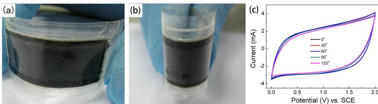
**Fig. S11**(a,b) Digital photographs of the as-fabricated asymmetric supercapacitor device. The images demonstrate the high flexibility of the device. Even after repeated twisting there is no obvious harm to its structural integrity. (c) CV curves of asymmetric supercapacitor under different bending angle.
