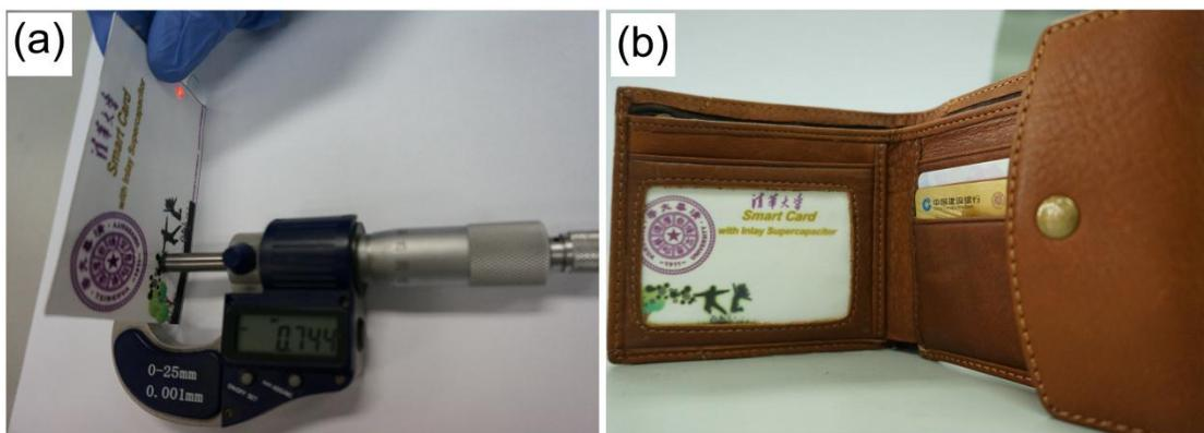
**Fig.S15** (a) A photograph which shows the thickness measurement of smart card with inlay supercapacitors. (b) The photograph which shows the smart card in a wallet. The total thickness is 0.77mm which is thinner than the commercial credit card. The supercapacitor based electronic can be wearable.
