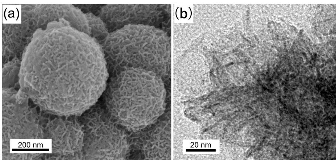
**Fig. S3** (a) SEM and (b) TEM images of the  $\text{MnO}_2/\text{PEDOT:PSS}$  electrode. The  $\text{MnO}_2/\text{PEDOT:PSS}$  nanospheres have rough surface textures which increase the total surface of the active materials. Because of the water-solubility of PEDOT:PSS and  $\text{MnO}_2$ , aqueous electrolyte can be fully immersed in the active substance.
