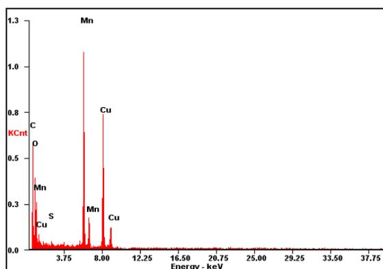
**Fig. S4** EDAX spectrum of MnO<sub>2</sub>/PEDOT:PSS. The spectrum of the nanocomposite containing signals from C, O, Mn and S further confirm the existence of MnO<sub>2</sub> and PEDOT:PSS.
