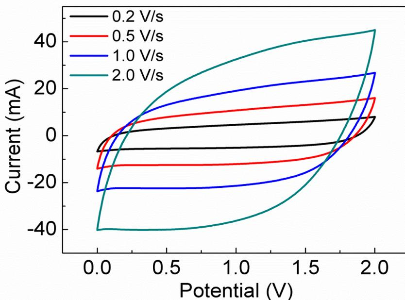
**Fig. S8** CV curves of (MnO<sub>2</sub>/PEDOT:PSS)/AC supercapacitor at scan rate of 0.2, 0.5, 1.0, 2.0V/s. Even at high scan rate of 2.0V/s, the CV curve still remains good rectangle indicates the excellent rate capability of the asymmetric supercapacitor.
