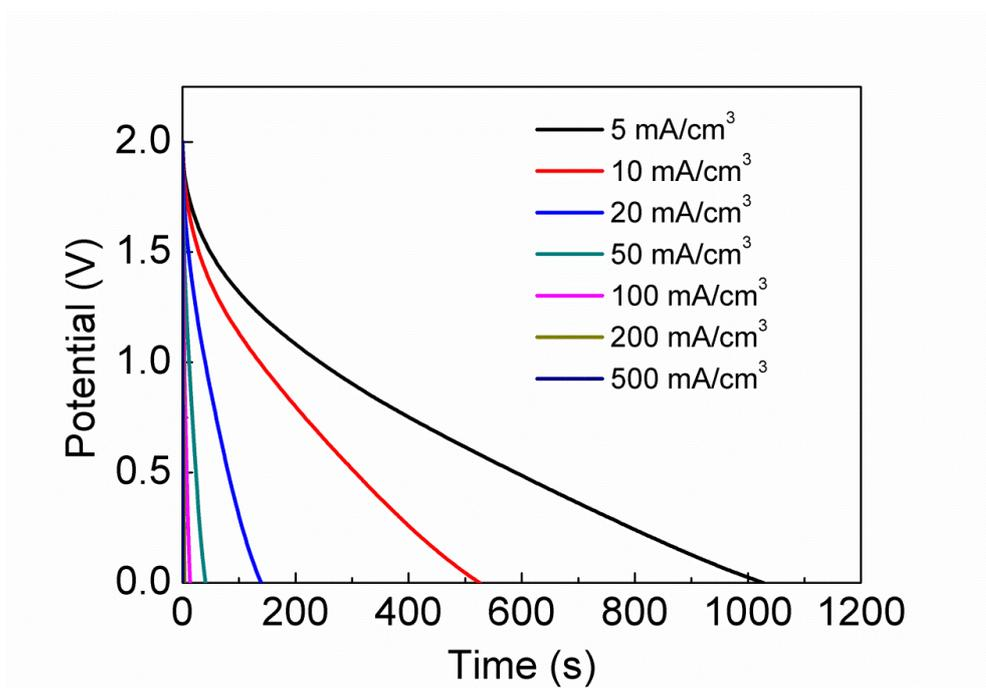
**Fig. S10** Discharging curves of the MnO<sub>2</sub>/AC asymmetric supercapacitor at different current density from 5 to 500 mA/cm<sup>3</sup>
