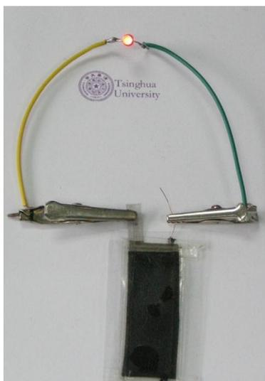
**Fig. S12** A photograph showing that the asymmetric supercapacitor can lighten up a red LED indicator (1.8 V, 20 mA). After charging for 13 s, the potential can be maintained as high as 2.0V.
