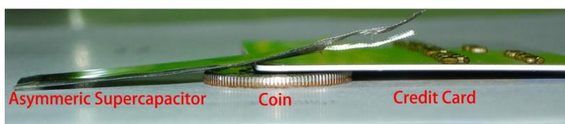
**Fig. S13** A photograph comparing the thickness of asymmetric supercapacitor, a coin (US quarter dollar) and a credit card. The as fabricated asymmetric supercapacitor is light-weight and as thin as 0.144mm, which is much thinner than that of coin and credit card.
