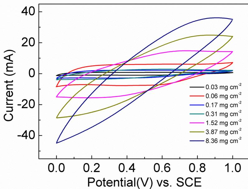
**Fig. S6** CV curves of MnO<sub>2</sub>/PEDOT:PSS with different deposition times at scan rates of 20 mV/s, respectively.
