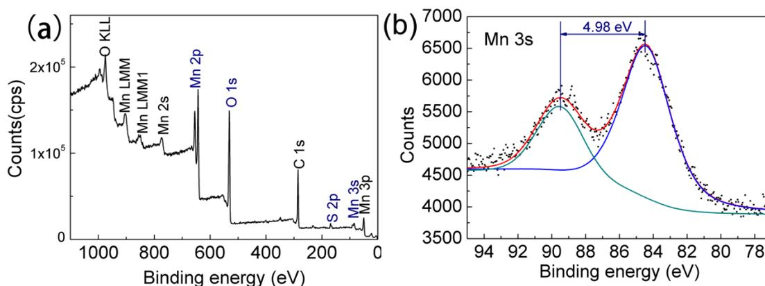
**Fig. S5** (a) Surface scanning XPS full spectrum of the MnO<sub>2</sub>/PEDOT:PSS composite. The XPS full spectrum containing signals from Mn, O, S and C elements indicates the presence of both MnO<sub>2</sub> and PEDOT:PSS. (b) Mn 3s core level XPS spectrum of MnO<sub>2</sub>/PEDOT:PSS.
