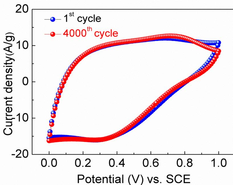
**Fig. S7** The CV curves of 1<sup>st</sup> and 4000<sup>th</sup> cycles of MnO<sub>2</sub>/PEDOT:PSS electrode at scan rate of 50mV/s. The CV curves are almost overlapped which indicates the excellent cycle performance.
