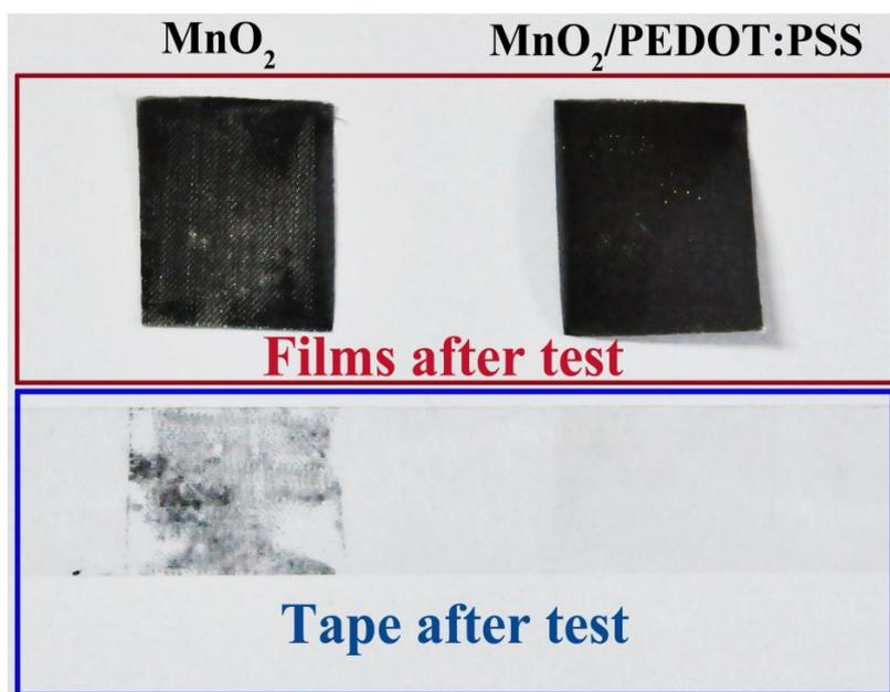
**Fig. S2** Tape method is used for adhesion test. The  $\text{MnO}_2$  films are prepared without PEDOT:PSS (left) and with PEDOT:PSS (right). The tape after the test is shown in the blue box. Tape tested for  $\text{MnO}_2/\text{PEDOT:PSS}$  electrode (right) shows no noticeable residues while that for  $\text{MnO}_2$  electrode exhibits a significant amount of powder residues that are detached from the electrode.
