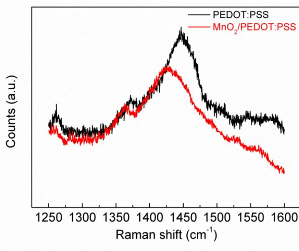
**Fig. S1** Counts vs. Raman shift of PEDOT:PSS and MnO<sub>2</sub>/PEDOT:PSS composite electrode.
