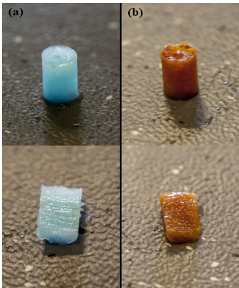
Figure S3: Photographs of whole MHCMPs containing two different metal hydroxides (upper row), and their cross-sections (lower row): (a) copper (II) hydroxide, (b) iron (III)-aluminium hydroxide. The different MHCMPs were produced using a single cycle with 0.4 M salt solutions.
