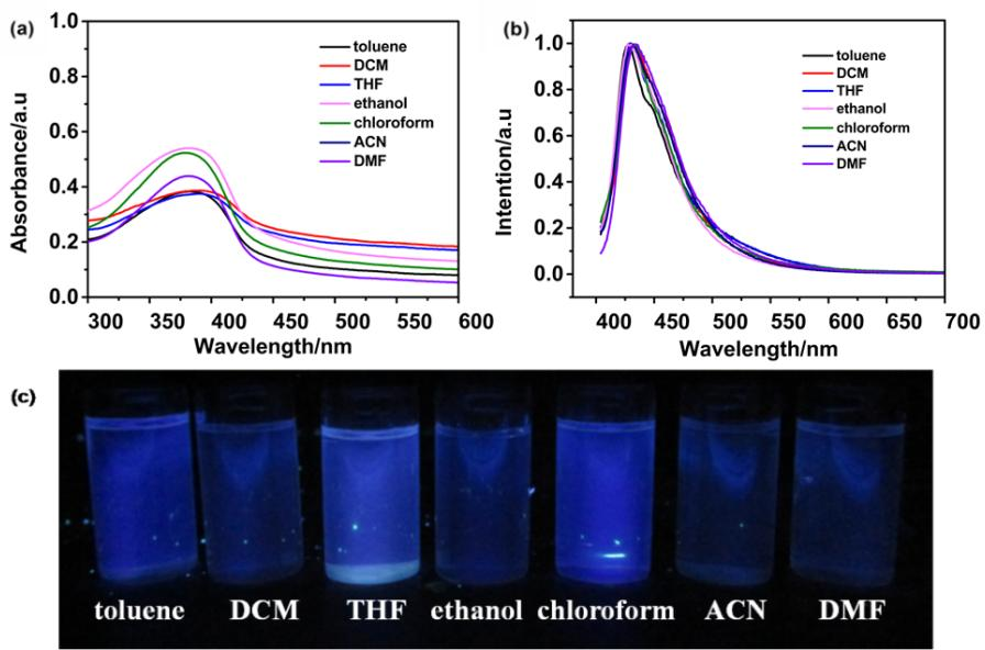
**Fig. S4** (a) UV-vis and (b) Normalized fluorescence ( $\lambda_{\text{ex}} = 386 \text{ nm}$ ) of **NN-ph**; (c) Luminescence photographs of **NN-ph** in different solvents under UV irradiation ( $\lambda_{\text{ex}} = 365 \text{ nm}$ ).
