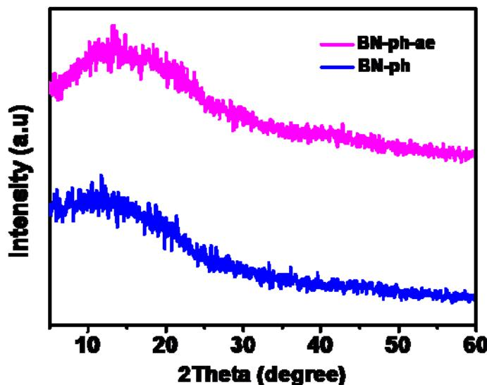
**Fig. S1** (a) XRD pattern of BN-ph and BN-ph-ae
