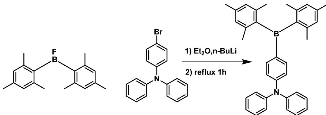
To the solution of 4-bromo-N, N-diphenylaniline (0.5 g, 1.54 mmol) in dry Et<sub>2</sub>O (30 mL) added n-BuLi (1.62 mmol, 1.6 M) at RT. After 10 min stirring, solution of Mes<sub>2</sub>BF (0.83 g, 3.09 mmol) in Et<sub>2</sub>O
