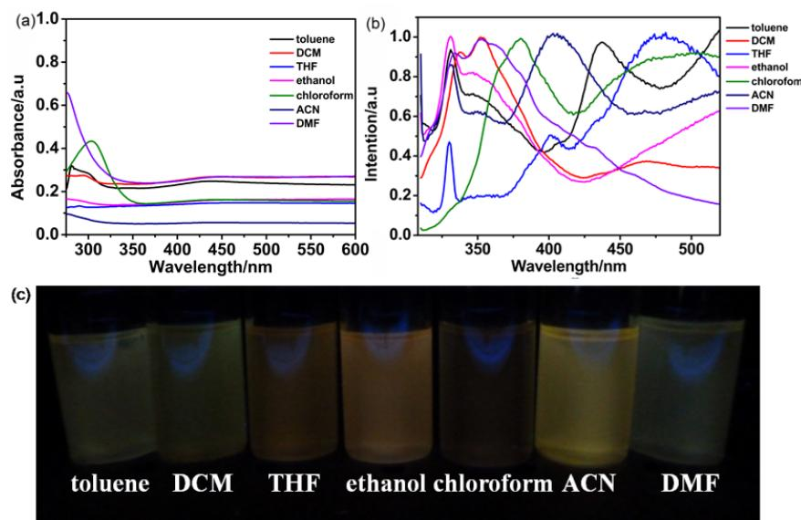
**Fig. S3** (a) UV-vis and (b) Normalized fluorescence ( $\lambda_{\text{ex}} = 300 \text{ nm}$ ) of **BN-ph-ae**; (c) Luminescence photographs of **BN-ph-ae** in different solvents under UV irradiation ( $\lambda_{\text{ex}} = 365 \text{ nm}$ ).
