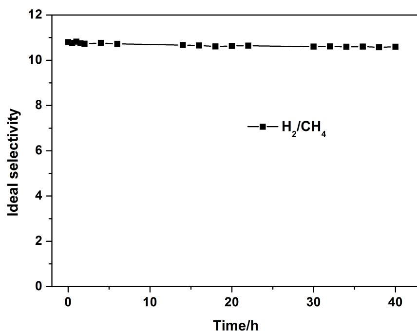
**Fig. S5** Ideal  $\text{H}_2/\text{CH}_4$  separation factor as-synthesized ZIF-8 membrane as a function of time at room temperature and feed pressure of 1 bar.
