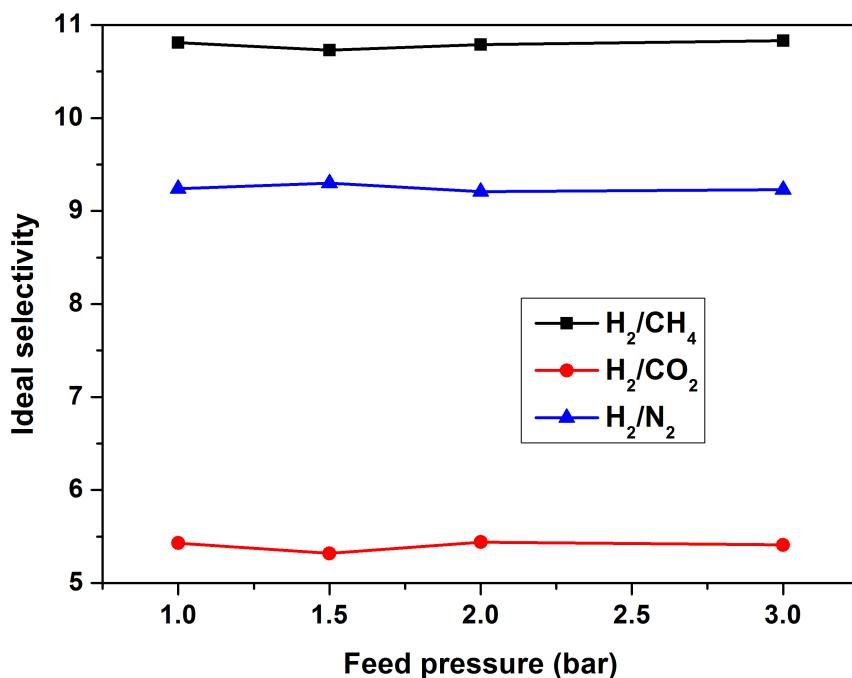
**Fig. S3** The ideal selectivity of as-synthesized ZIF-8 membrane as a function of feed pressure at room temperature.
