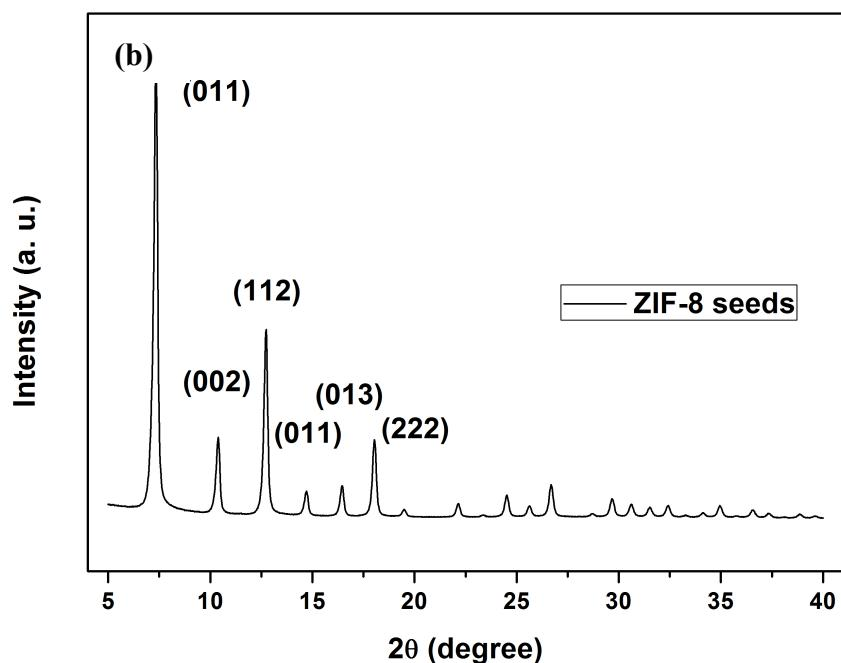
**Fig. S1.** SEM image (a) and XRD pattern (b) of pure ZIF-8 seeds.
