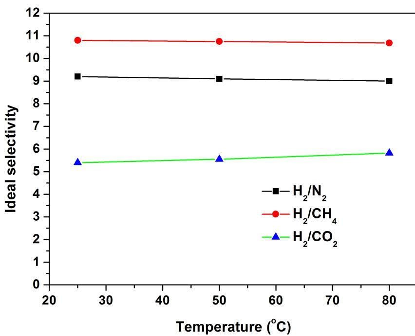
**Fig. S4** The ideal selectivity of as-synthesized ZIF-8 membrane as a function of temperature at feed pressure of 1 bar.
