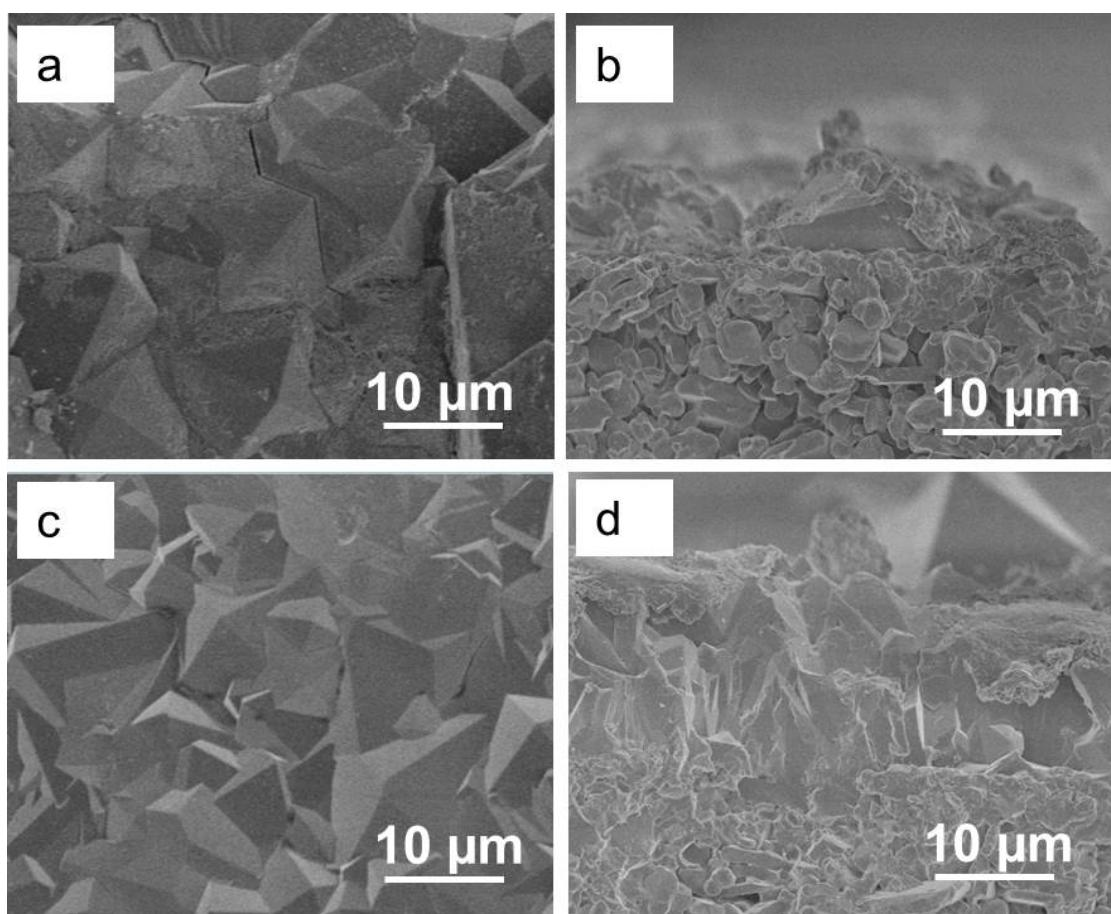
**Fig. S2** SEM image of ZIF-8 membranes synthesized with different seeding methods: a,b: dip-coating and e,f: hot dip-coating (ZIF-8 content: 0.5 wt%); a,c: top-view; b,d,:
