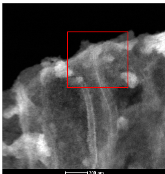
Fig. S2 STEM image of Graphene/TiO 2 /S nanocomposite.
