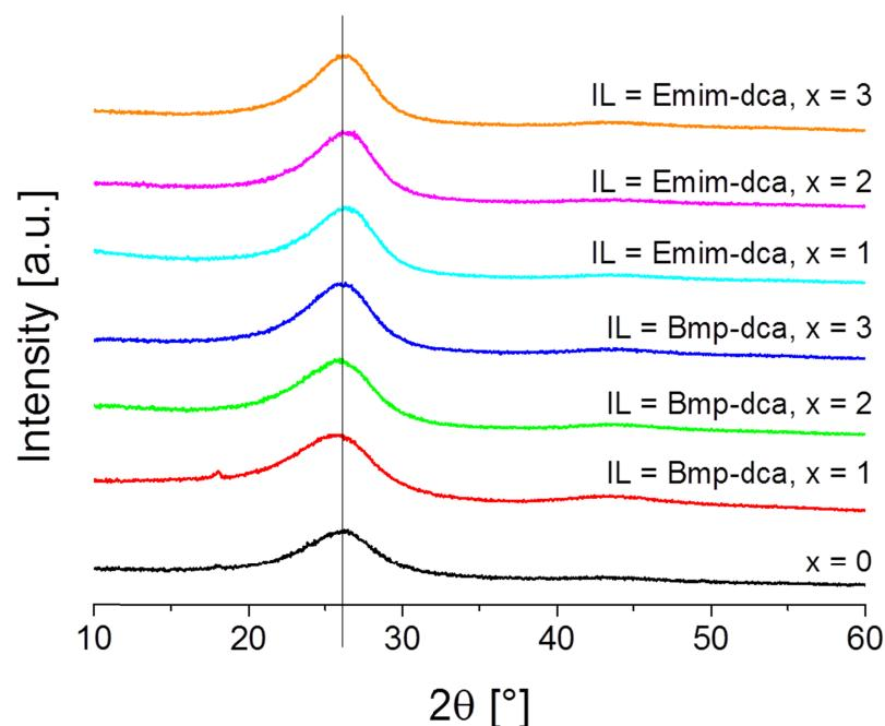
**Figure SI-3** XRD patterns of N-S-dC\_IL\_x\_800.
