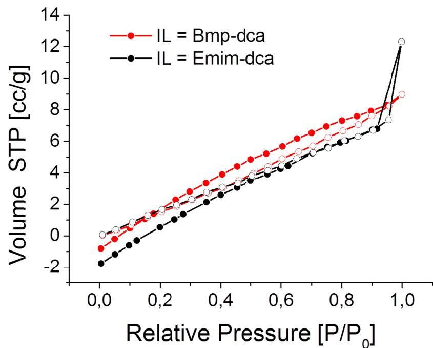
**Figure SI-7** Nitrogen sorption isotherms N-S-dC\_IL\_2\_800 with IL=Emim-dca (black) and Bmp-dca (red).
