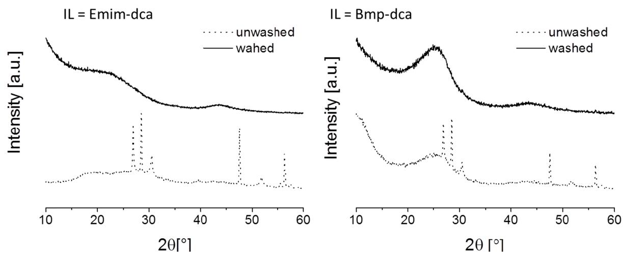
**Figure SI-8** XRD patterns of N-S-dC\_IL\_2\_SZ\_3\_800 with IL=Emim-dca (left) and IL=Bmp-dca (right) before (dotted) and after (solid) washing with HCl.
