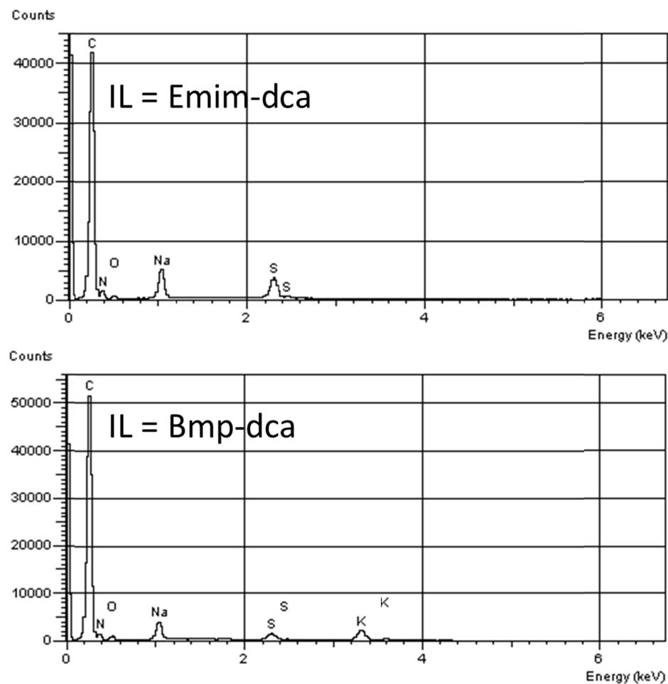
**Figure SI-4** EDX of N-S-dC\_IL\_2\_800 with IL=Emim-dca (top) and Bmp-dca (bottom).
