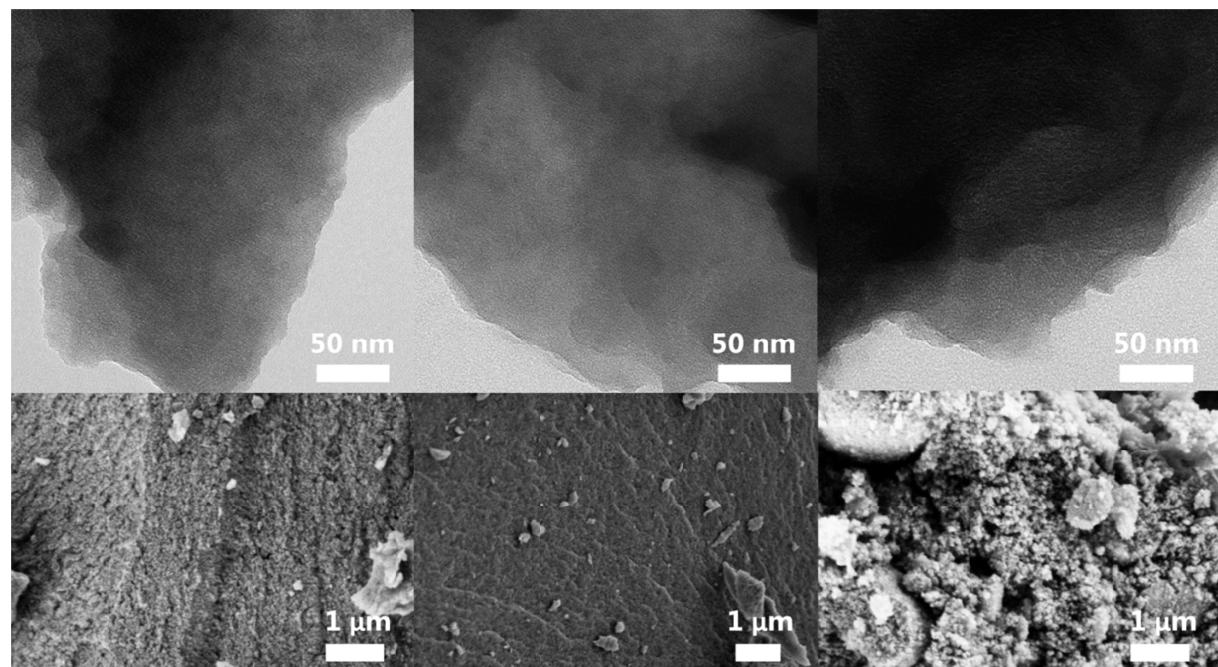
**Figure SI-6** TEM (top) and SEM (bottom) of N-S-dC\_Bmp-dca\_x\_800 with  $x=1$  (left),  $2$  (middle) and  $3$  (right).
