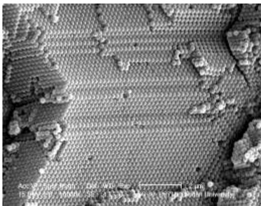
**Figure S1.** SEM micrograph of the PS template to prepare three dimensional (3D)-ordered macroporous  $\text{LiFePO}_4$ .
