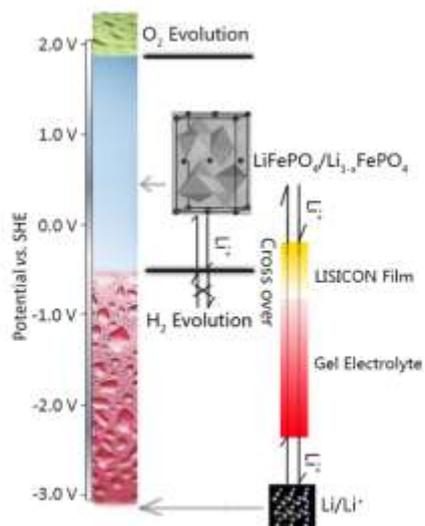
**Figure S3** Schematic illustration of the “cross-over” effect of  $\text{Li}^+$  ions in the composite coating.
