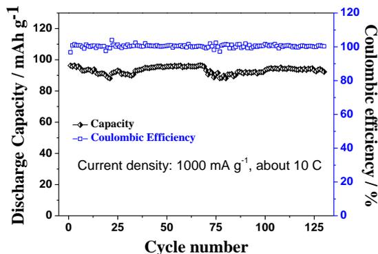
**Figure S2.** Cycling behaviour of the  $\text{LiFePO}_4$  cathode in  $0.5 \text{ mol l}^{-1} \text{Li}_2\text{SO}_4$  aqueous solution at the current density of  $1000 \text{ mA g}^{-1}$ .
