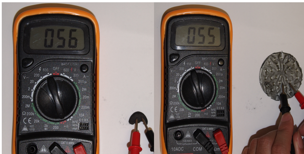
Fig.5S Resistance test of CNS-800 (left) and reduced graphene film reduced by HI (right) using a multimeter
