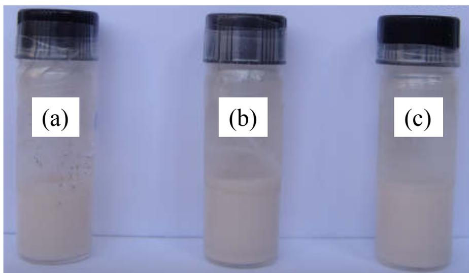
**Fig. S3.** Dispersion of 1 (a), 2 (b) and 5 (c) wt% of 2 in 2 mL of THF with after 168 h.
