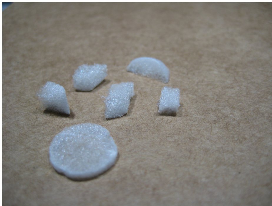
Figure S1. 0.5 CNF aerogel ( 8.1 \text{ mg/cm}^3 ) from freezing at -20^\circ\text{C} could be cut into various shapes (thin disc, square, trapezoid and wedges) by a sharp razor without appreciable deformation.
