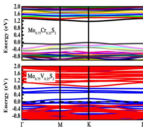
**Fig. S3** The calculated band structures of  $\text{Mo}_{0.75}\text{V}_{0.25}\text{S}_2$  and  $\text{Mo}_{0.75}\text{Cr}_{0.25}\text{S}_2$  with DFT+U ( $U=5.95\text{eV}$ ,  $J=0.95\text{eV}$ ). The calculated band gap of  $\text{Mo}_{0.75}\text{Cr}_{0.25}\text{S}_2$  is about 1.2 eV.
