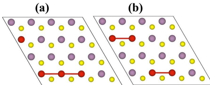
**Fig. S1** Two additional configurations of  $\text{Mo}_{0.75}\text{Cr}_{0.25}\text{S}_2$  considered for checking reliability of SQS: (a) three T atoms connected in a straight line and (b) two parallel pairs of neighboring T atoms.
