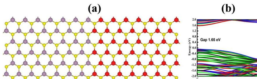
**Fig. S2** The atomic structure (a) and band structure (b) of armchair  $\text{MoS}_2\text{-WS}_2$  heterostructure with the strip width of 22 Å, as mentioned in the context.
