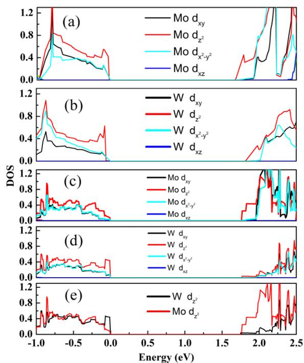
**Fig. S4** Projected density of states (PDOS) of  $d$  orbitals for pure  $\text{MoS}_2$  (a), pure  $\text{WS}_2$  (b) and heterostructure of armchair  $\text{MoS}_2$ - $\text{WS}_2$  (The width of the strip is  $12.7 \text{ \AA}$ , which corresponds to AHS) (c) and (d) show the PDOS of Mo and W atoms of heterostructure. (e) shows the  $d_{z^2}$  of both Mo and W atoms in heterostructure.
