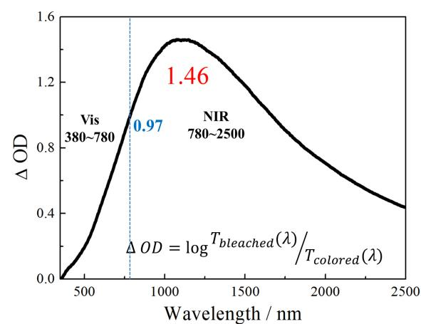
Fig.4S. Optical density change of mesoporous WO<sub>3</sub>-based device
