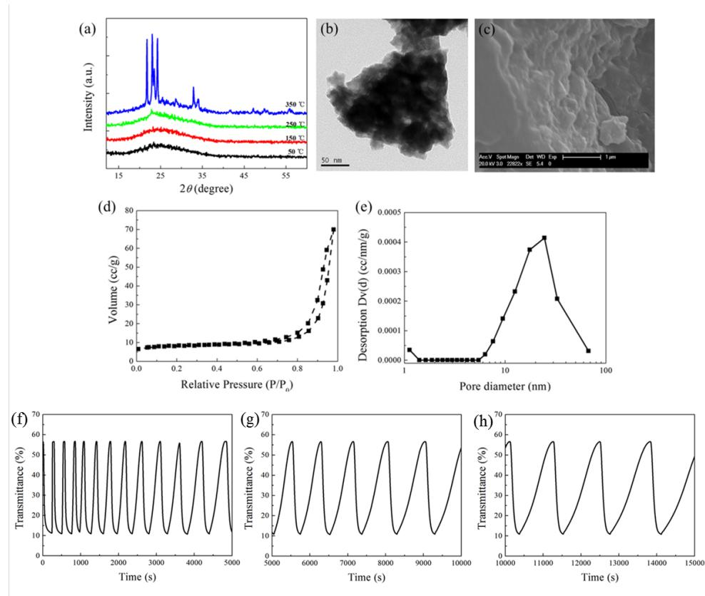
Fig. 6S Crystallinity and morphology of the standard  $\text{WO}_3$  film (a) XRD; (b) TEM; (c) SEM; the representative N<sub>2</sub> desorption isotherms (d) and pore size distribution (e); as well as the corresponding coloring/bleaching behaviors (f) ~ (h)
