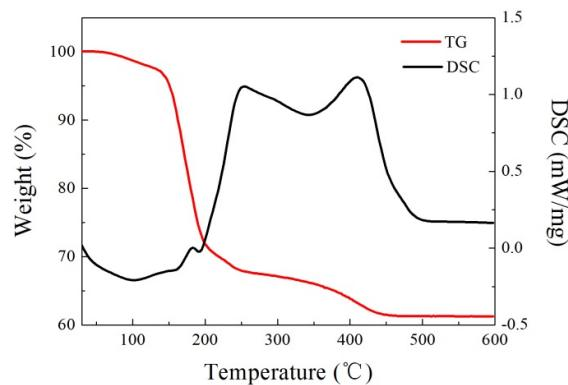
Fig.1S. TG-DSC curves of the PTA/F127 xerogel powder
