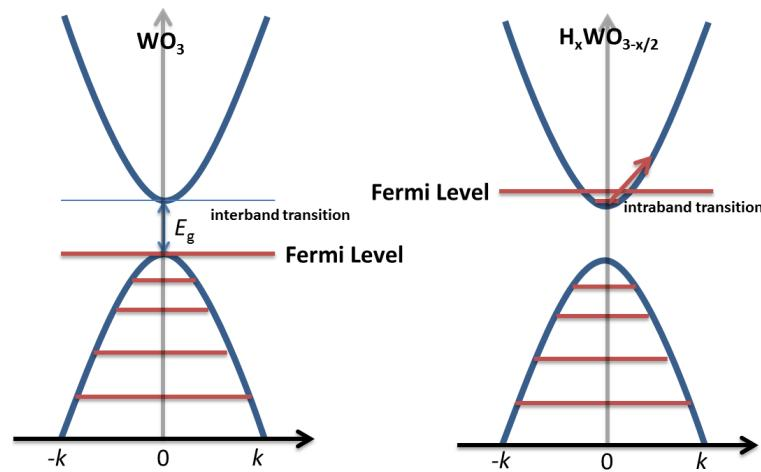
Fig. 5S Schematic of the band structures for  $\text{WO}_3$  (bleached) and  $\text{H}_x\text{WO}_{3-x/2}$  (colored)
