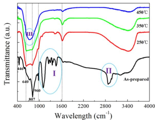
Fig.2S. FT-IR spectra of the hybrid films annealed at different temperatures
