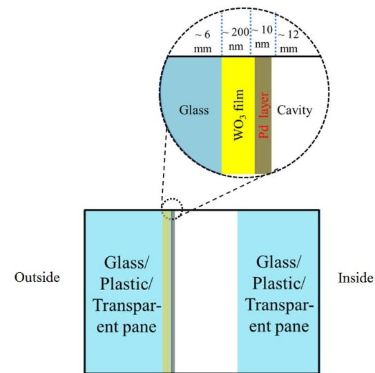
Fig.3S. Schematic of the gasochromic device
