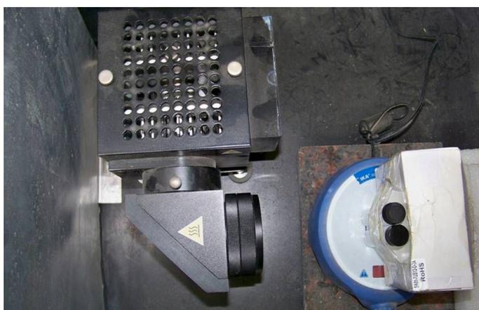
**Fig. S3** Photograph of the experimental setup for photocatalytic oxidation of alcohols into corresponding aldehydes.
