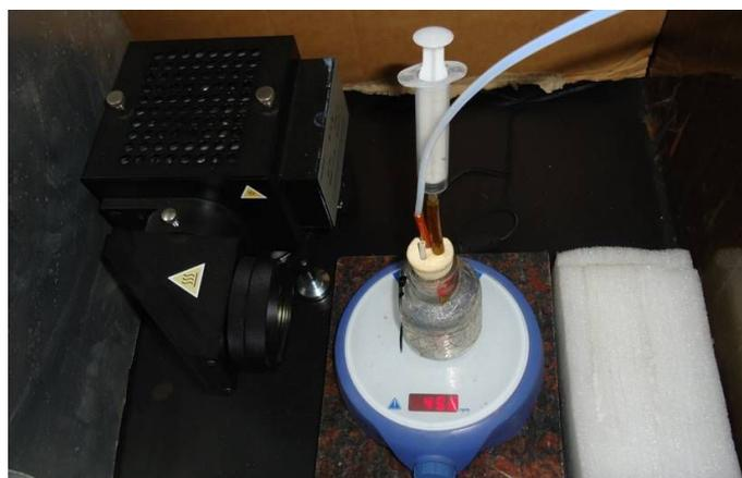
**Fig. S1** Photograph of the experimental setup for photocatalytic reduction of nitroaromatic compounds.
