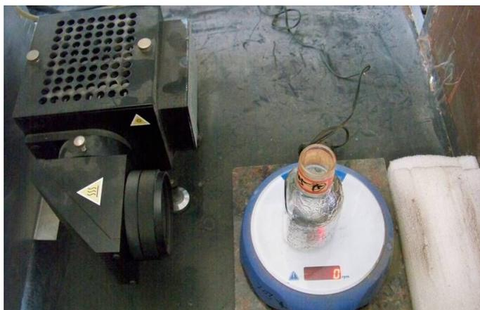
**Fig. S2** Photograph of the experimental setup for photocatalytic reduction of Cr (VI).
