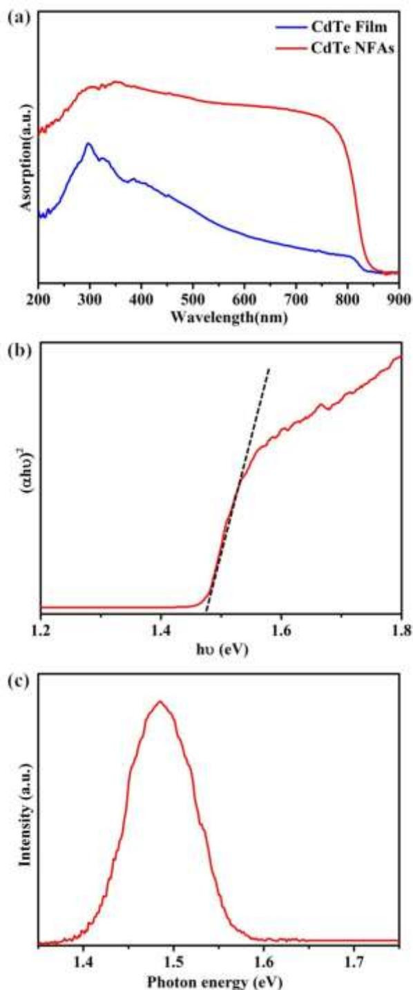
**Figure S7.** (a) Absorption spectra of CdTe film and NFAs obtained by PIH at 350 and 420 °C, respectively. (b)  $(\alpha h\nu)^2$ - $h\nu$  plot according to the absorption spectrum of NFAs in (a), extrapolation of the linear part till its intersection with the  $h\nu$ -axis gives the value band gap. (c) PL spectrum of the CdTe NFAs on FTO substrate.
