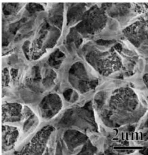
**Figure S5.** SEM image of the product obtained by PIH at 350 °C .
