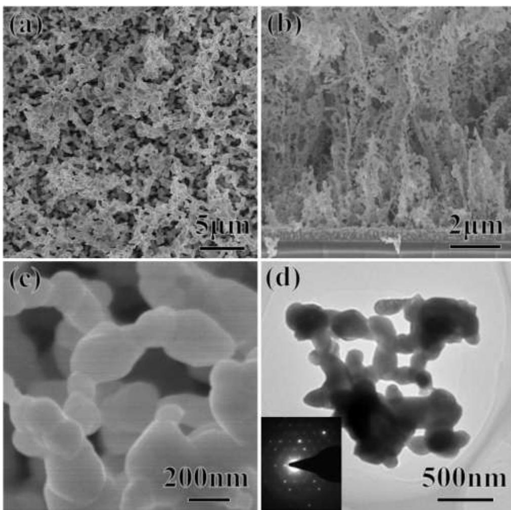
**Figure S6.** Characterizations of the product obtained by PIH at 450 °C. (a) Top-down, (b) cross-section , and (c) high magnification SEM images, (d) TEM image, inset is the SAED pattern.
