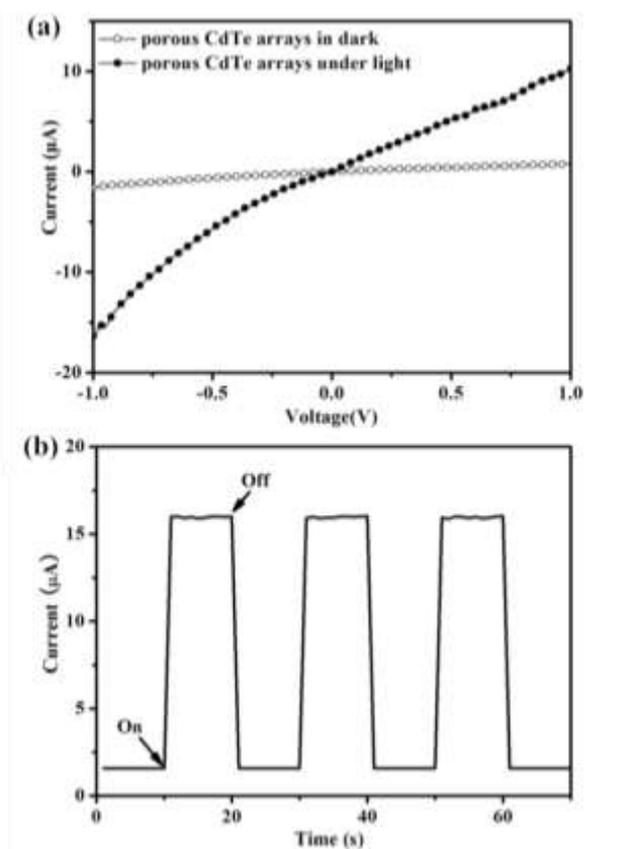
**Figure S8.** Photoresponse of porous CdTe arrays on FTO substrate. (a) I-V curves measured in dark and under white light illumination, respectively. (b) On-off cycles at a constant bias of -1.0 V.
