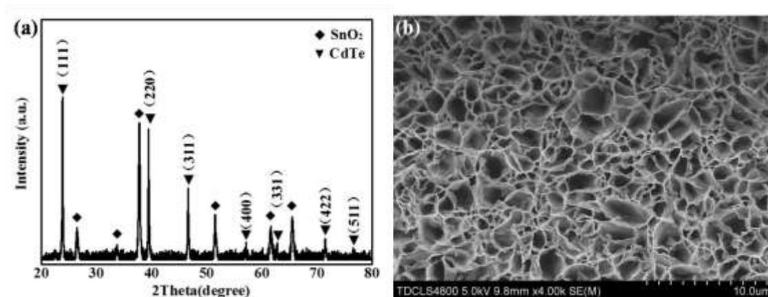
**Figure S2.** (a) XRD pattern and (b) SEM image of CdTe nanoflakes obtained by PIH at 420 °C for 5 min.
