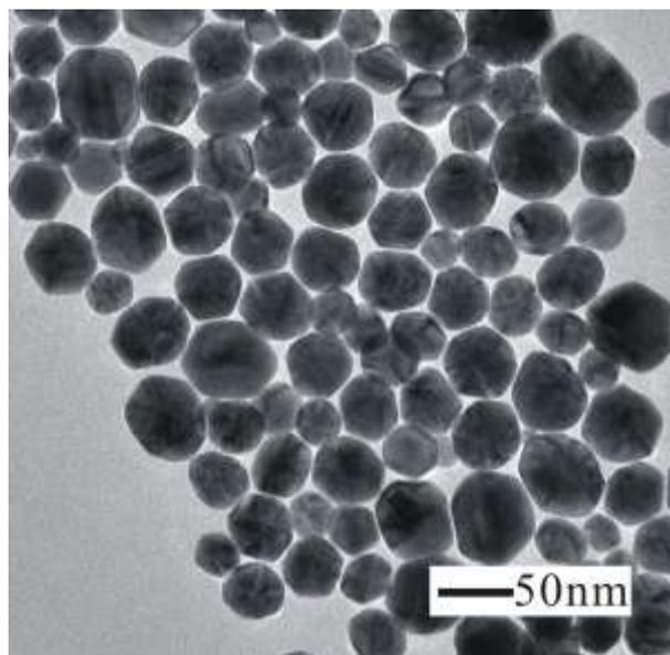
Figure S6. The TEM image of Au particles prepared under the standard procedure but without the addition of Cu micro-particles.
