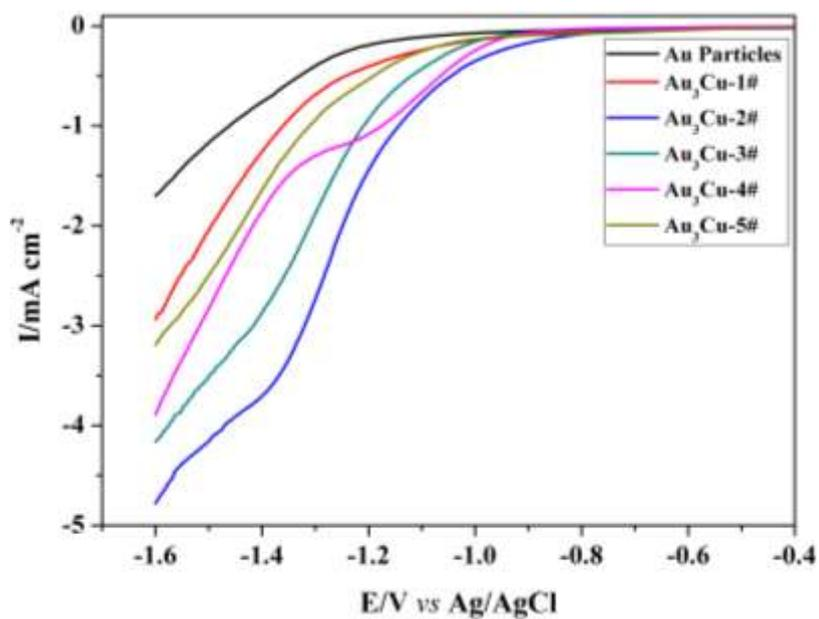
Figure S7. Electroreduction performance of Au<sub>3</sub>Cu NCs and Au nanoparticles in N<sub>2</sub>-saturated PBS solution.
