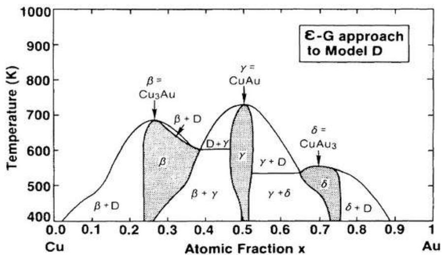
Figure S1. The phase diagram of Au-Cu at different atom ratios.
