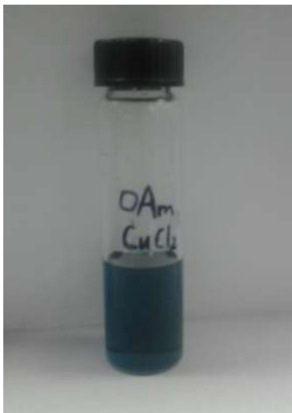
Figure S3. A photograph of the  $\text{Cu}^{2+}$ -based complex, formed by adding 20 mg  $\text{CuCl}_2$  into the solution of oleylamine and heated for 6h under  $200^\circ\text{C}$ .
