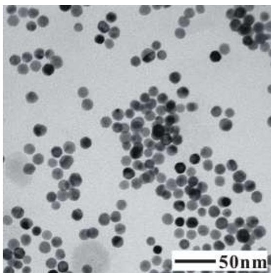
Figure S5. TEM image of the Au<sub>3</sub>Cu NCs prepared using the standard procedure except that the Cu micro-particles were replaced by CuCl<sub>2</sub>.
