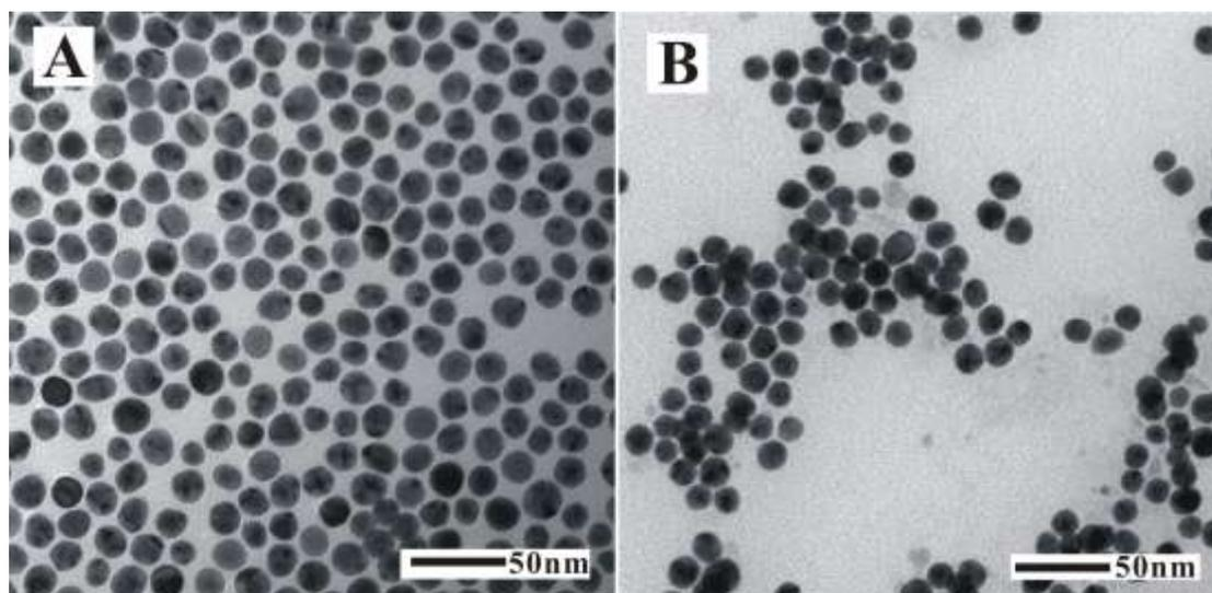
Figure S4. (A) TEM image of Au NCs that were used as seeds; (B) TEM image of the product that were prepared using the standard procedure except that the  $\text{AuPPh}_3\text{Cl}$  and Cu micro-particles were replaced by presynthesized Au NCs and  $\text{CuCl}_2$ , respectively.
