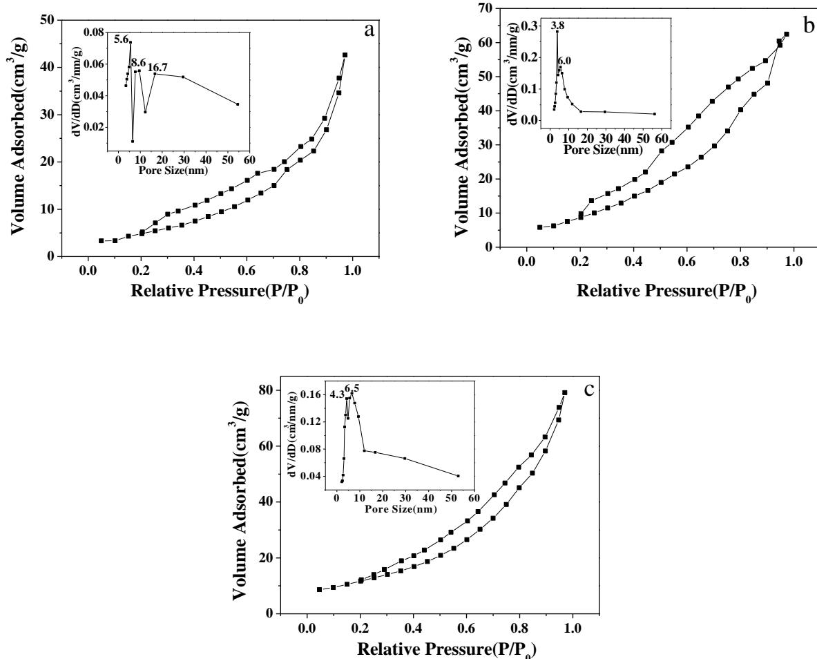
Fig. S4 Typical N<sub>2</sub> adsorption-desorption isotherm and pore-size distribution curve (inset) of the mesoporous Al<sub>2</sub>O<sub>3</sub>-In<sub>2</sub>O<sub>3</sub> composited NFs with different atomic ratios.
