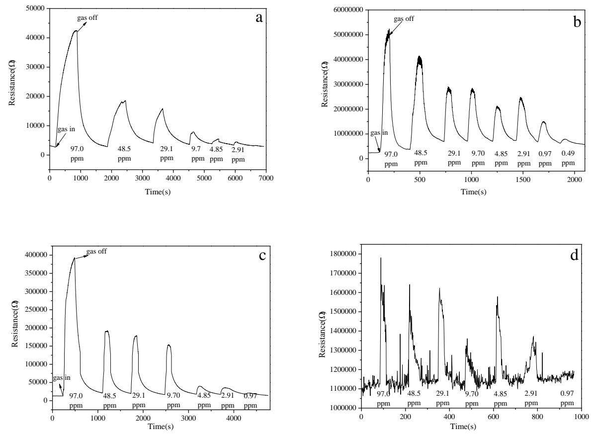
Fig. S2 Dynamic response-recovery curves of Al<sub>2</sub>O<sub>3</sub>-In<sub>2</sub>O<sub>3</sub> composites NFs thin film sensors with different atomic ratios to 0.49-97 ppm NO<sub>x</sub> at room temperature (RT) in air. (a) Pure In<sub>2</sub>O<sub>3</sub> NTs, (b) Meso-15Al NTs, (c) Meso-25Al NRs, (d) Porous pure Al<sub>2</sub>O<sub>3</sub> NRs (RH: 42%).
