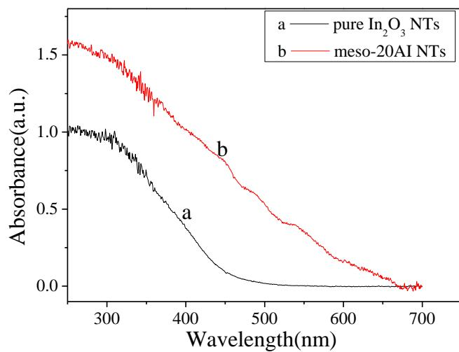
Fig. S5 UV-vis diffuse absorption spectra of Al<sub>2</sub>O<sub>3</sub>-In<sub>2</sub>O<sub>3</sub> composites NTs with different atomic ratios.
