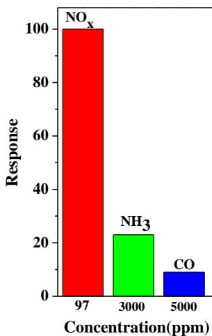
Fig. S3 The meso-20AI NTs thin film sensor with response to various gases at RT in air (RH: 42 %)
