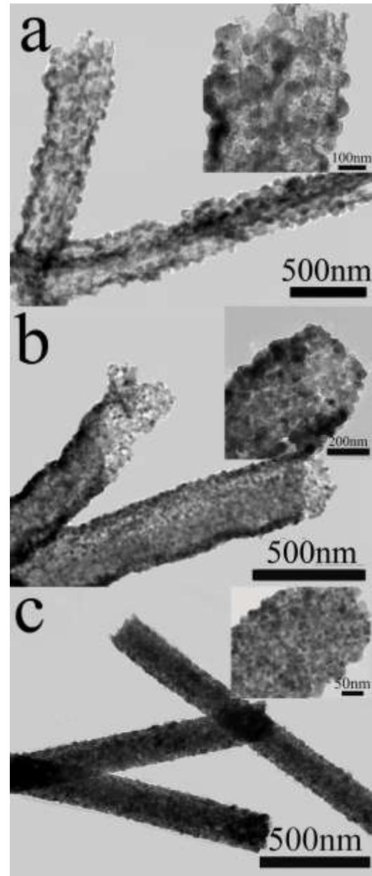
Fig. S1 TEM images of  $\text{Al}_2\text{O}_3$ - $\text{In}_2\text{O}_3$  composites with different atomic ratios
