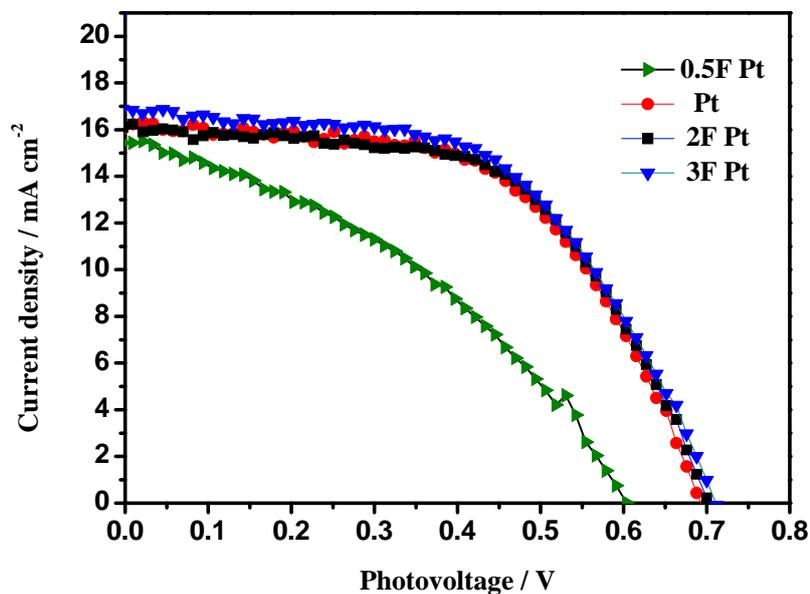
**Fig. S1** The  $J$ - $V$  curves of the DSCs with different folds of the mass of the conventional Pt.
