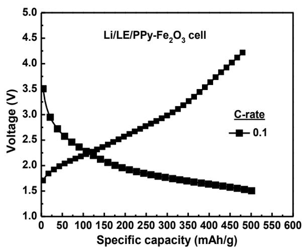
**Figure S7.** Initial charge-discharge capacity of Li /PPy-Fe<sub>2</sub>O<sub>3</sub> cells with liquid electrolyte (0.1 C-rate, RT).
