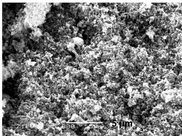
**Figure S3.** SEM image of  $\gamma$ -Fe<sub>2</sub>O<sub>3</sub>-PPy core-shell.
