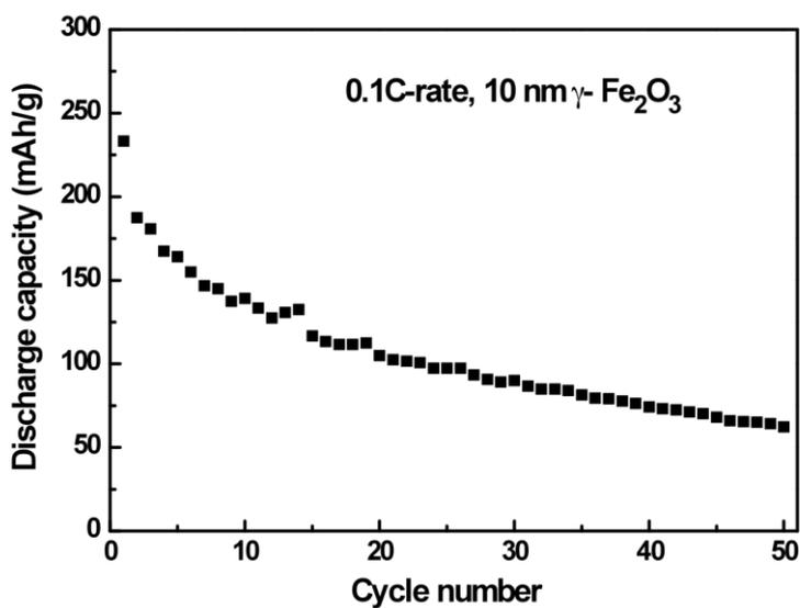
**Figure S6.** Cycle performance of nano sized  $\gamma$ -Fe<sub>2</sub>O<sub>3</sub> cell at 0.1C-rate (Room temperature).
