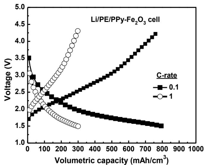
**Figure S4.** Initial charge-discharge volumetric capacities of Li/GPE/PPy-Fe<sub>2</sub>O<sub>3</sub> cells at different current densities (0.1 and 1 C-rate, RT).
