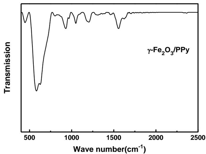
**Figure S1.** FT-IR pattern of  $\gamma\text{-Fe}_2\text{O}_3\text{-PPy}$  core-shell.
