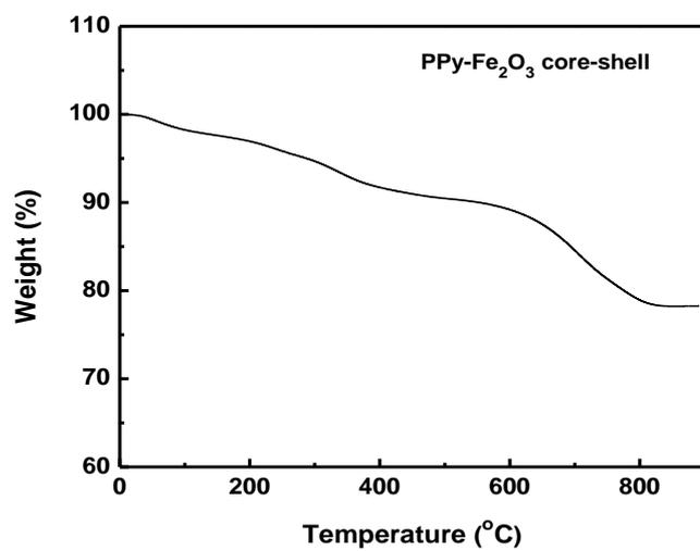
**Figure S2.** TGA curve of  $\gamma\text{-Fe}_2\text{O}_3\text{-PPy}$  core-shell.
