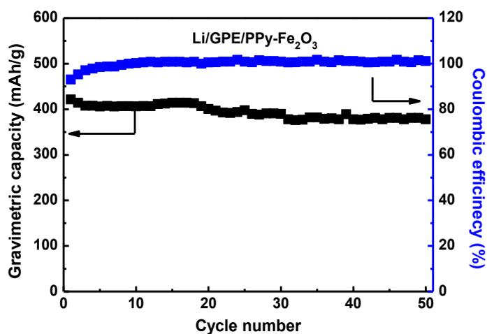
**Figure S5.** Cycle performance and coulombic efficiency of Li/GPE/PPy-Fe<sub>2</sub>O<sub>3</sub> cells at 0.1C-rate (Room temperature).
