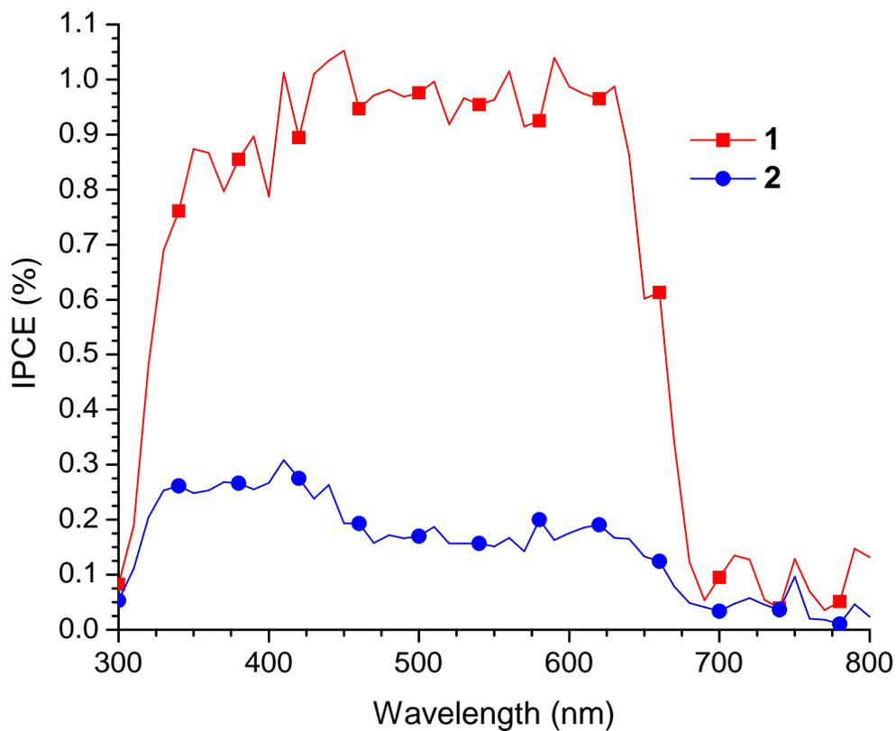
**Fig. S2** IPCE spectra of the most efficient BHJ solar cells based on active layers of P3HT:1–2 (10:8 by mass). All devices were based on the ITO/PEDOT:PSS/P3HT:1 or 2/LiF/Al architecture.
