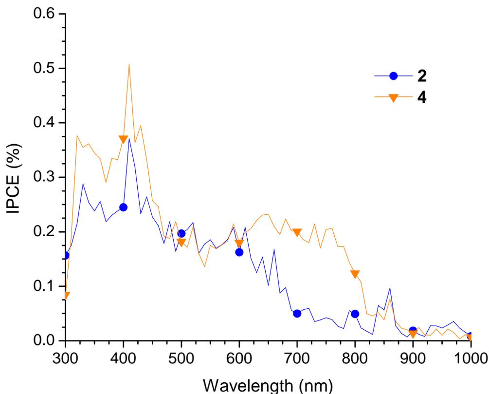
**Fig. S3** IPCE spectra of the most efficient BHJ solar cells based on active layers of **2** or **4**:PC<sub>61</sub>BM (60:40 by mass). All devices were based on the ITO/PEDOT:PSS/**2** or **4**:PC<sub>61</sub>BM/LiF/Al architecture.
