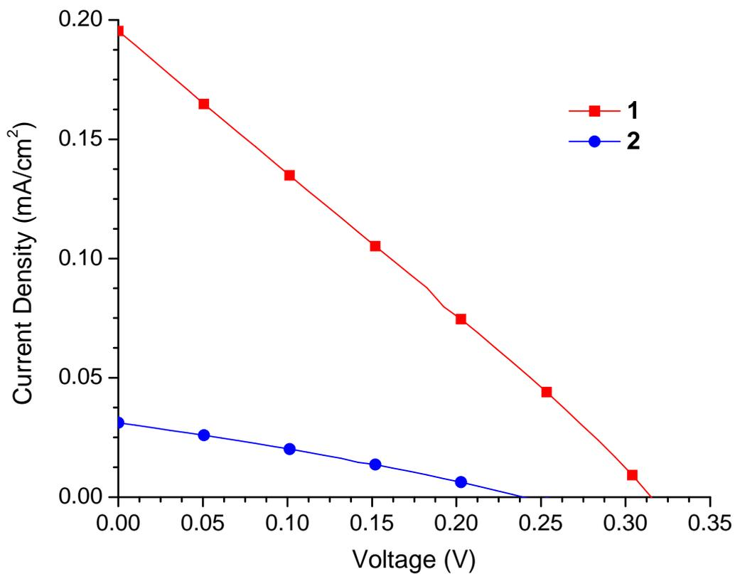
**Fig. S1** Current-voltage curves for the most efficient BJJ solar cells based on active layers of P3HT:1-2 (10:8 by mass). All devices were based on the ITO/PEDOT:PSS/P3HT:1 or 2/LiF/Al architecture.
