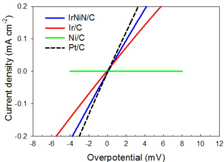
**Fig. S3** The *i*- $\eta$  plot at small  $\eta$  showing that the net current is linearly related to overpotential.
