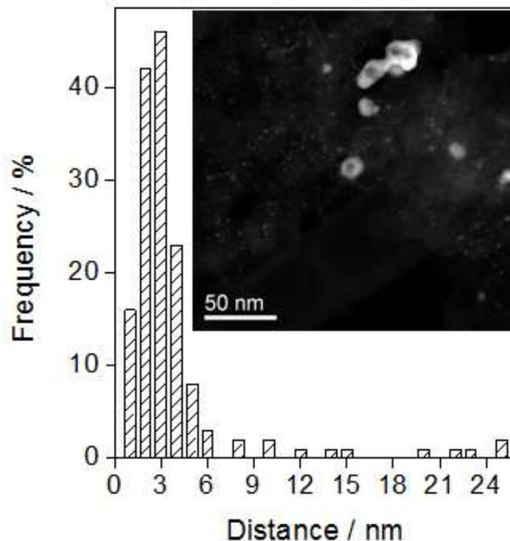
**Fig. S4** Particle size distribution of IrNiN core-shell nanoparticles (sample size=150).
