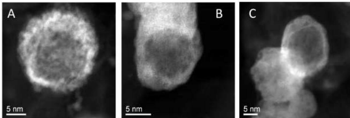
**Fig. S1** HAADF-STEM images of hollow IrNiN nanoparticles.
