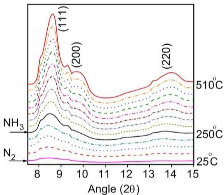
**Fig. S2** *In situ* synchrotron XRD patterns (the wavelength: 0.3184 Å) obtained from the IrNi<sub>3</sub> nanoparticles during reduction in N<sub>2</sub> and NH<sub>3</sub> flow at increasing temperatures.
