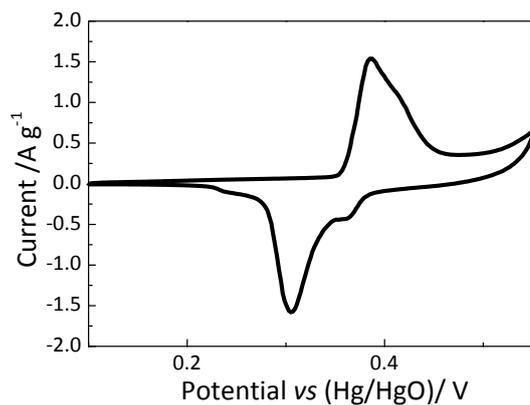
**Fig. S7** CV profiles of NiO electrode measured at a scan rate of 2 mV/s.
