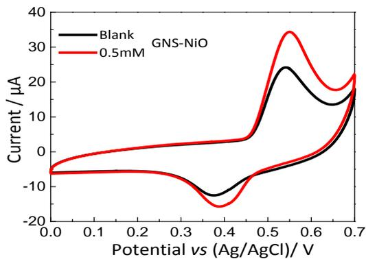
**Fig. S5** CV profiles of the GNS-NiO modified GC electrodes with and without glucose (0.5 mM) at  $50 \text{ mV s}^{-1}$ .
