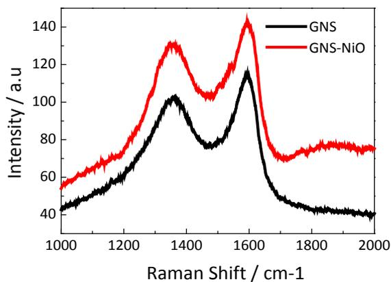
**Fig. S3** Raman spectra of the GNS-NiO hybrid and GNS.
