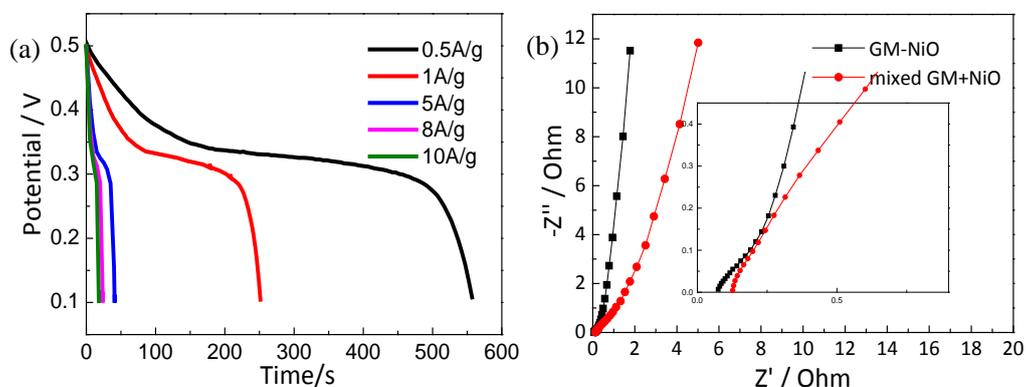
**Fig. S8** Electrochemical performance of the 3D GM-NiO electrodes measured in 6 M KOH solution. (a) Galvanostatic charge/discharge curves of GM-NiO hybrid electrode with different current densities. (b) Nyquist plots of GM-NiO hybrid and mixed GM+NiO electrodes.
