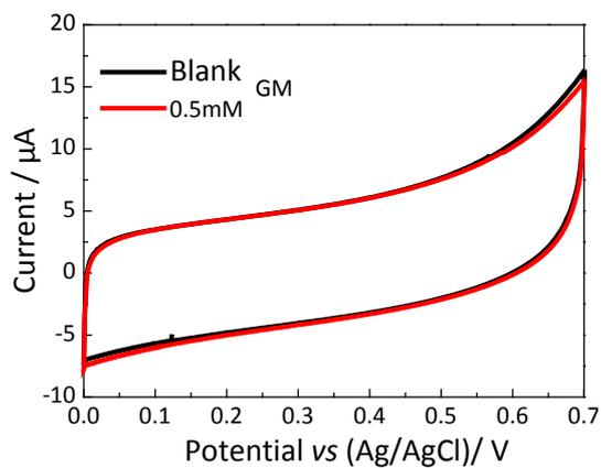
**Fig. S4** CV profiles of the GM modified GC electrodes with and without glucose (0.5 mM) at  $50 \text{ mV s}^{-1}$ . No peak is observed, indicating the GM has no activity towards the glucose.
