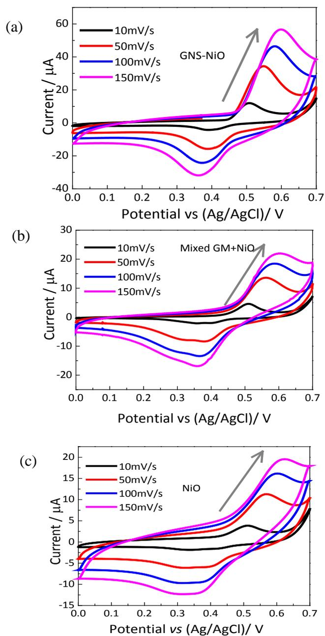
**Fig. S6** (a)-(c) show the CV profiles of the GNS-NiO hybrid, GM+NiO and NiO modified GC electrodes at different scan rates in the presence of 0.5 mM glucose.
