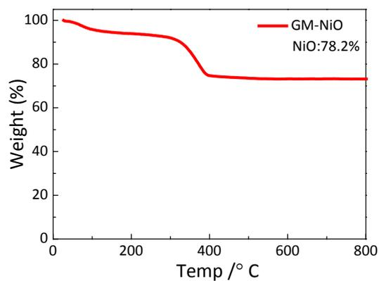
**Fig. S2** TG curve of the GM-NiO hybrid in the air atmosphere.
