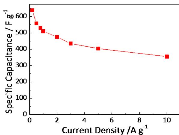
**Fig. S9** The capacitance of the single electrode based on the two-electrode measurement with different current densities.
