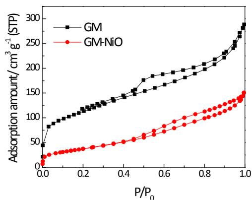
**Fig. S1** Nitrogen adsorption/desorption isotherms of GM-NiO hybrid and GM.
