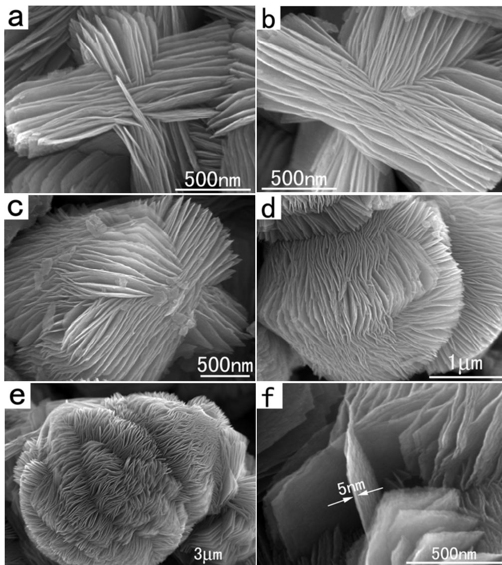
**Figure S5.** FESEM images of the more complex TiO<sub>2</sub> nanosheet superstructures obtained by extending reaction time: (a) 25 h, (b) 32 h, (c) 40 h, (d) 46 h, (e,f) 52 h.
