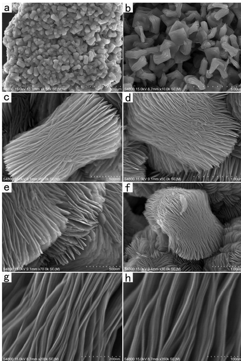
**Figure S4.** FESEM images of the TiO<sub>2</sub> nanosheet superstructures with different magnifications.
