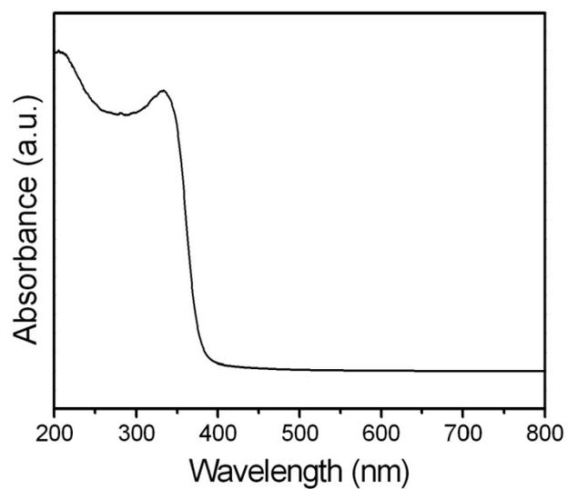
**Figure S3.** A typical UV-vis absorption spectrum of the anatase TiO<sub>2</sub> nanosheet superstructures.
