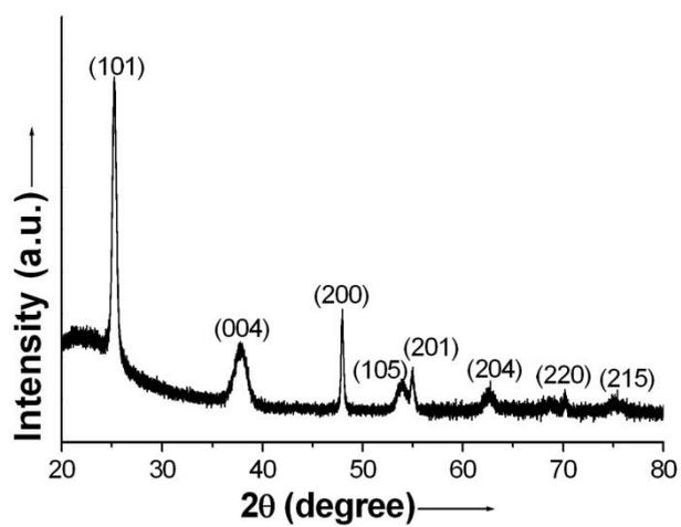
**Figure S8.** The XRD pattern of the sample after photocatalytic reaction.
