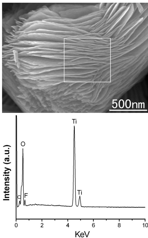
**Figure S1.** EDS spectrum of the as-synthesized large-scale, ultrathin, and (001) facets exposed anatase TiO<sub>2</sub> nanosheet superstructures.
