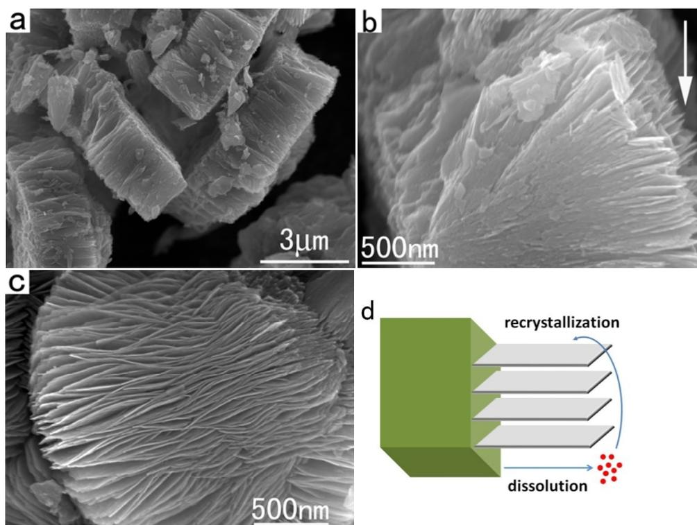
**Figure 6.** FESEM images of the samples recorded in different reaction times: a) 2 h, b) 8 h, and c) 18 h. d) Schematic illustration of the formation and shape evolution of the ultrathin TiO<sub>2</sub> nanosheet superstructures.
