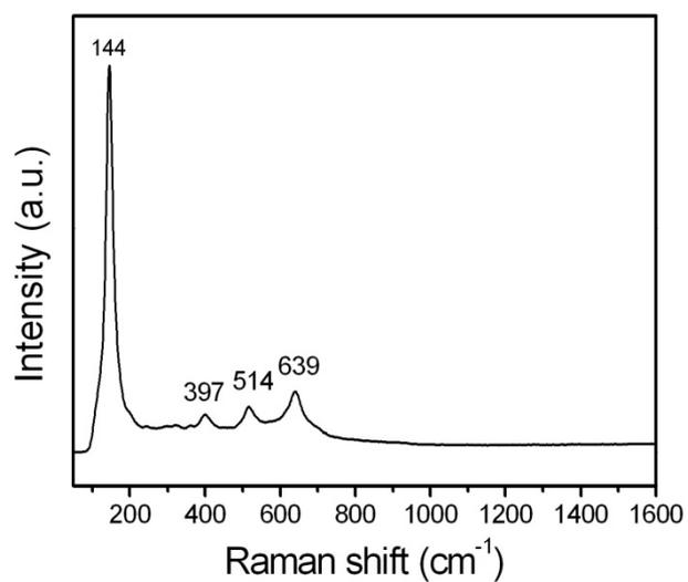
**Figure S2.** A typical Raman spectrum of the as-synthesized anatase TiO<sub>2</sub> nanosheet superstructures.
