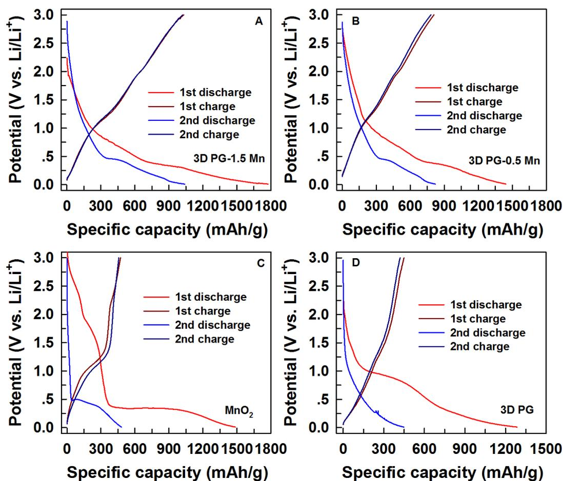
**Fig. S2** The galvanostatic discharge/charge profiles of various anode materials between 0.01 and 3 V at a current density of 100 mA h g<sup>-1</sup>.
