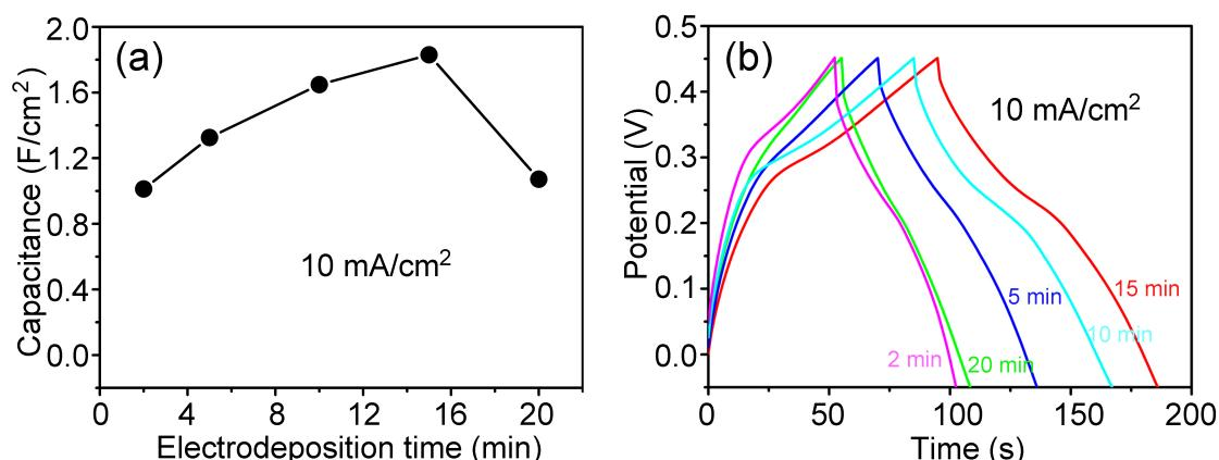
Figure S6. (a) Specific capacitance and (b) CD curves of the  $\text{NiCo}_2\text{O}_4@\text{MnO}_2$  electrode as a function of the  $\text{MnO}_2$  electrodeposition time.
