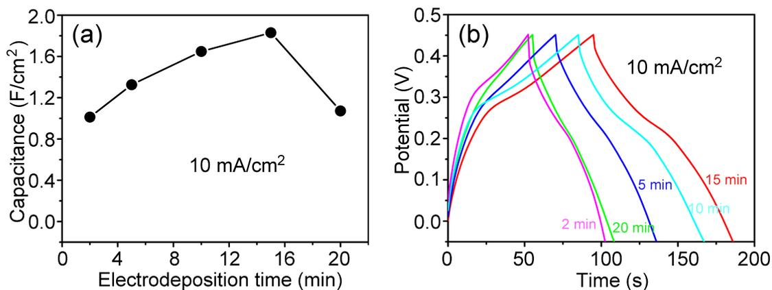
Figure S6. (a) Specific capacitance and (b) CD curves of the  $\text{NiCo}_2\text{O}_4@\text{MnO}_2$  electrode as a function of the  $\text{MnO}_2$  electrodeposition time.
