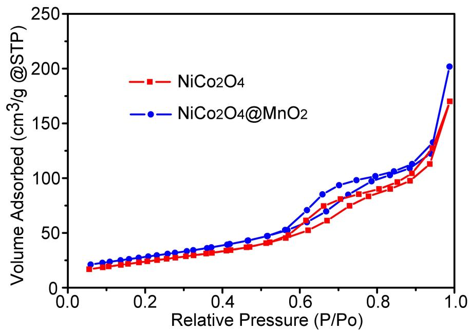
Figure S8. The BET surfaces of the  $\text{NiCo}_2\text{O}_4$  and  $\text{NiCo}_2\text{O}_4@\text{MnO}_2$ .
