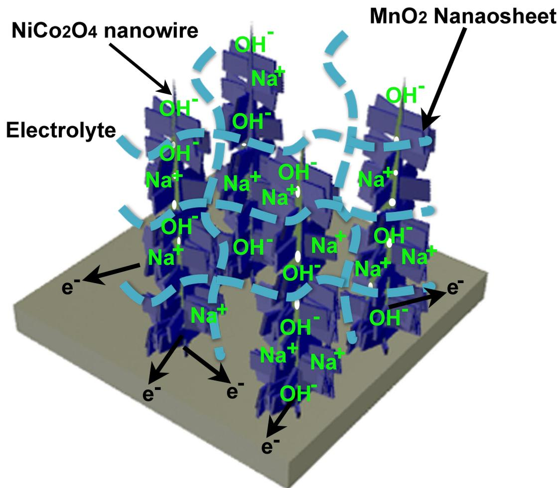
Figure S9. Schematic of the charge storage advantage of the hierarchical mesoporous  $\text{NiCo}_2\text{O}_4@ \text{MnO}_2$  core-shell nanowire arrays on Ni foam, in which both the  $\text{NiCo}_2\text{O}_4$  core and  $\text{MnO}_2$  shell materials contribute to the charge storage.
