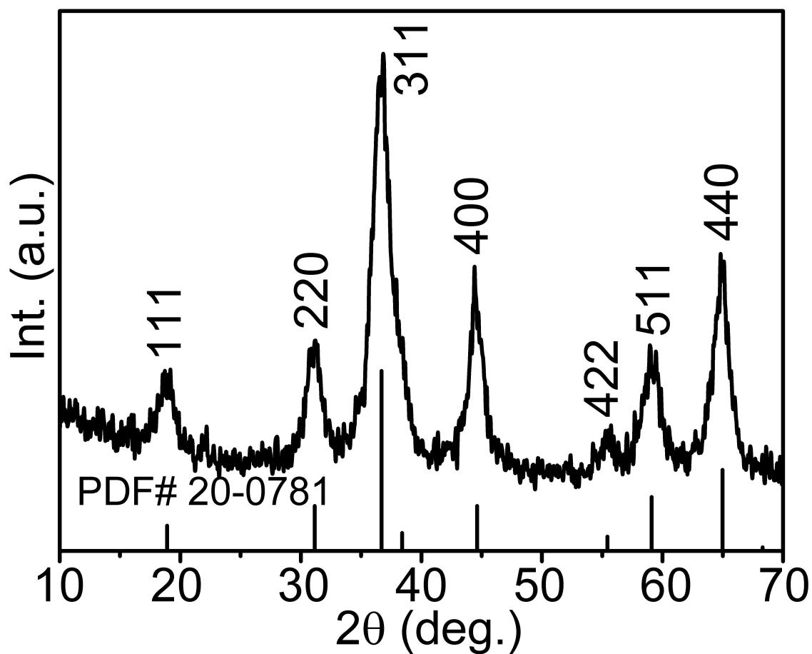
Figure S2. XRD pattern of the synthesized  $\text{NiCo}_2\text{O}_4$  material scratched from the Ni foam.
