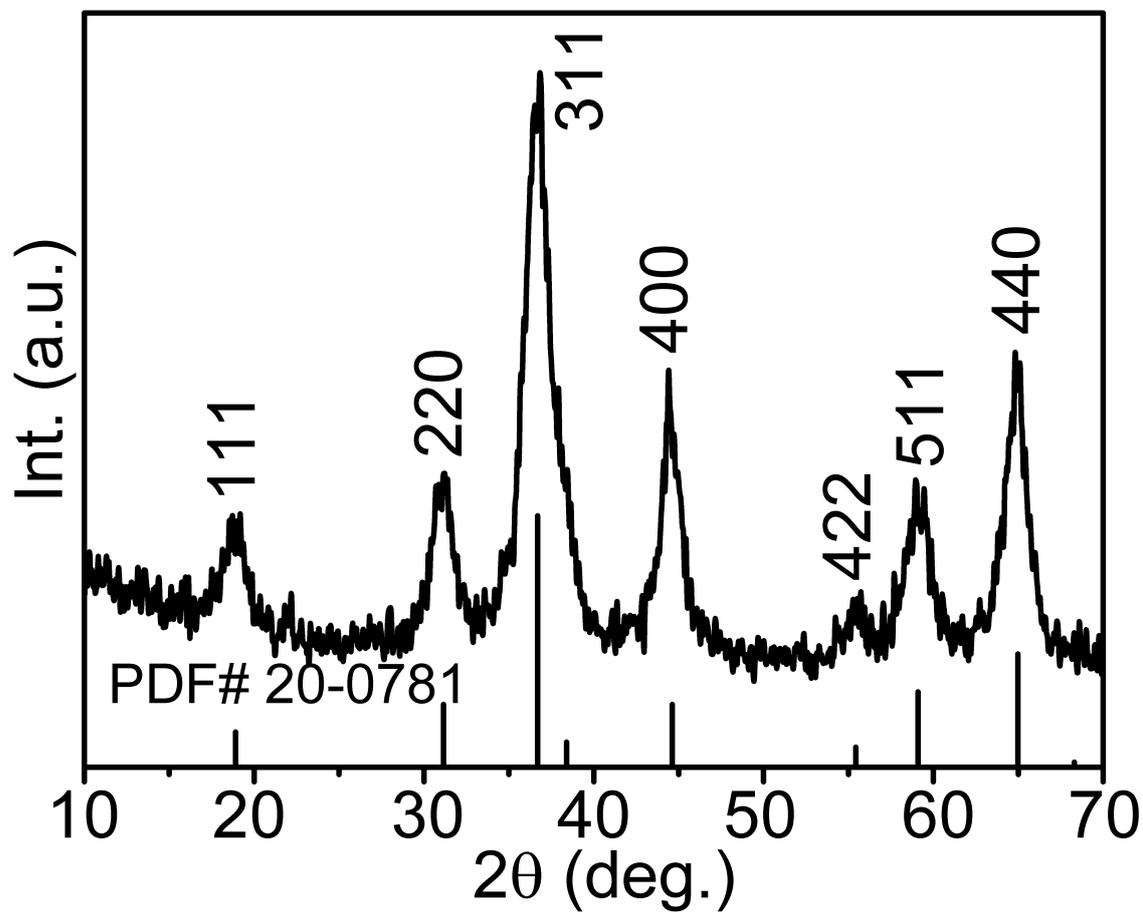
Figure S2. XRD pattern of the synthesized NiCo<sub>2</sub>O<sub>4</sub> material scratched from the Ni foam.
