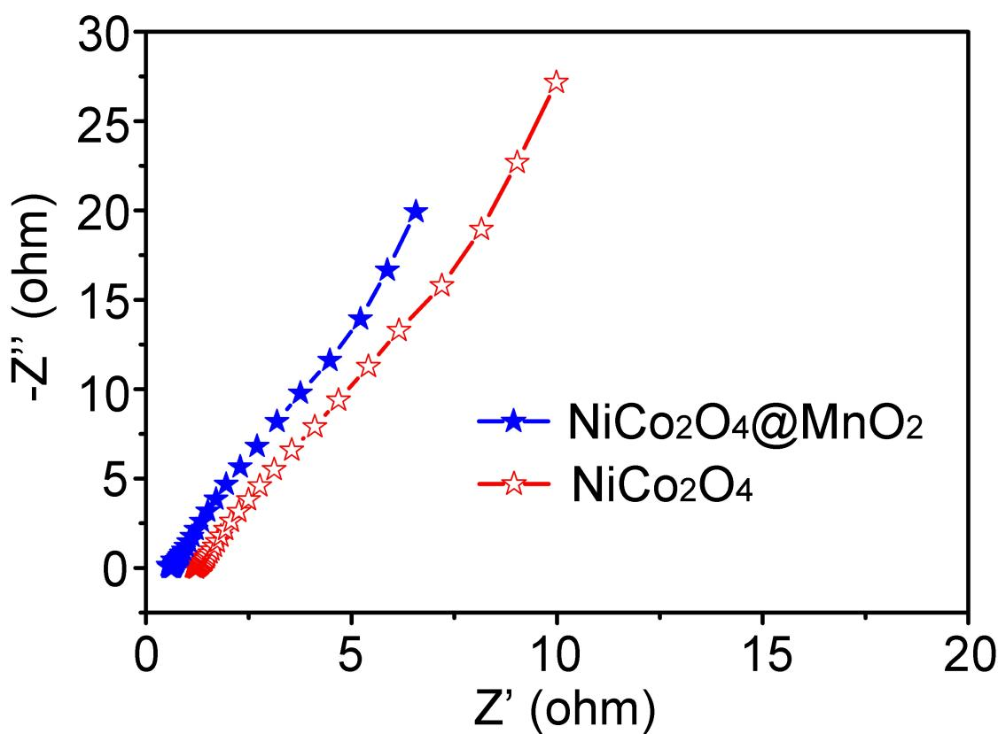
Figure S7. EIS spectra of the  $\text{NiCo}_2\text{O}_4@\text{MnO}_2$  and  $\text{NiCo}_2\text{O}_4$  electrode.
