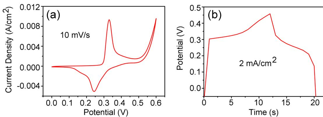
Figure S4. (a) CV and (a) CD curves of pure Ni foam.
