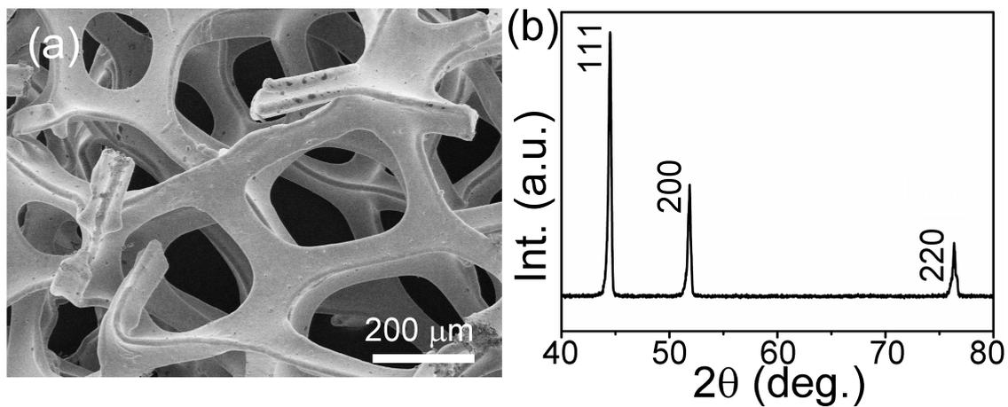
Figure S1. (a) SEM image and (b) XRD pattern of the treated Ni foam by HCl.
