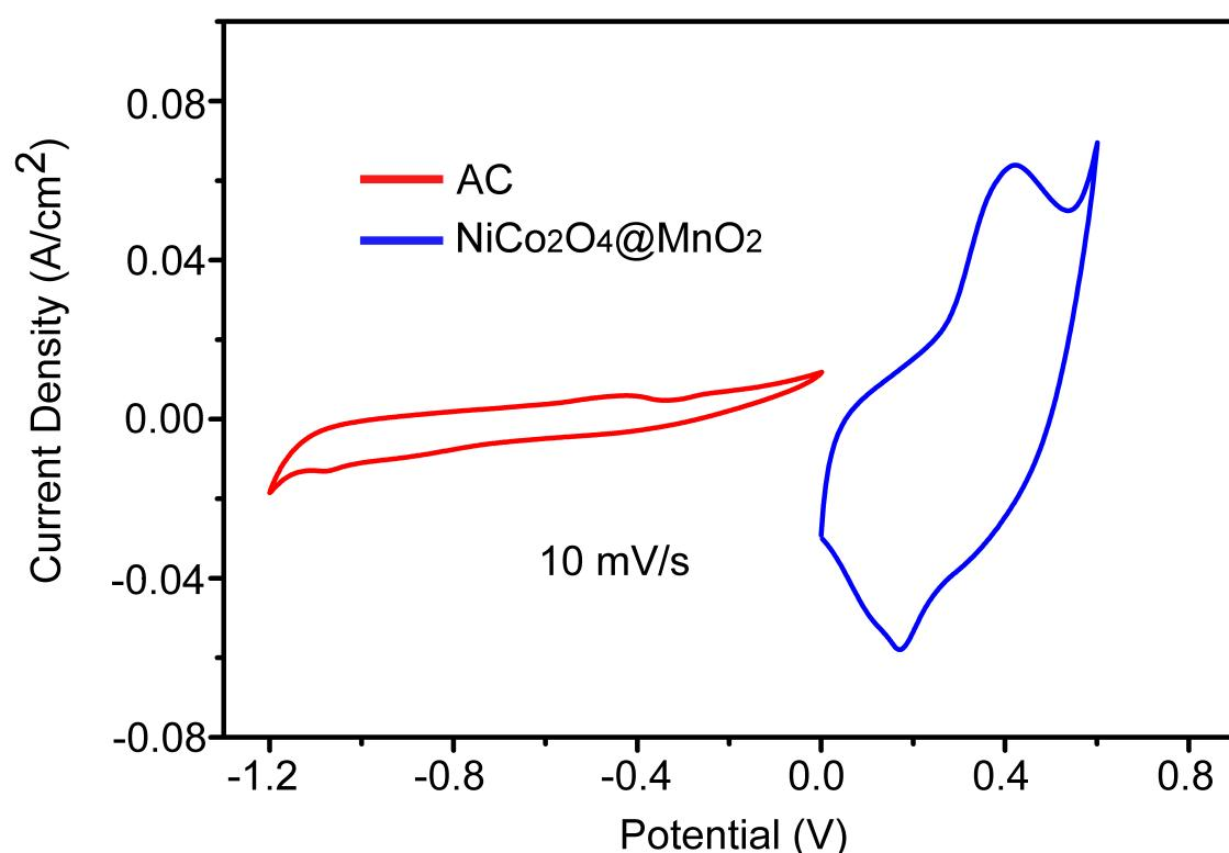
Figure S10. Comparative CV curves of the  $\text{NiCo}_2\text{O}_4@\text{MnO}_2$  and activated carbon (AC) electrodes performed in a three-electrode cell at 10 mV/s.
