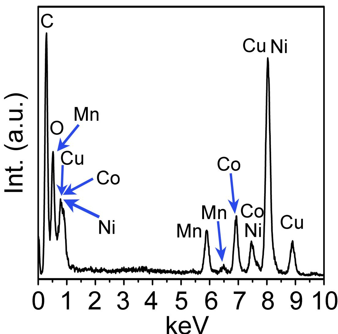
Figure S3. EDX spectrum of the hierarchical mesoporous  $\text{NiCo}_2\text{O}_4@\text{MnO}_2$  core-shell nanowires.
