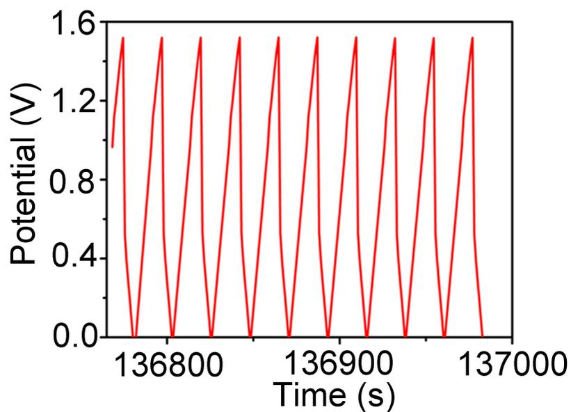
Figure S11. The CD curves of the last 10 cycles for the asymmetric supercapacitor.
