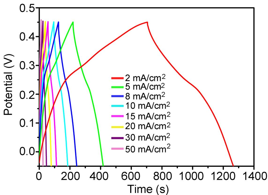
Figure S5. (a) CD curves of the  $\text{NiCo}_2\text{O}_4@\text{MnO}_2$  electrode at different current densities.
