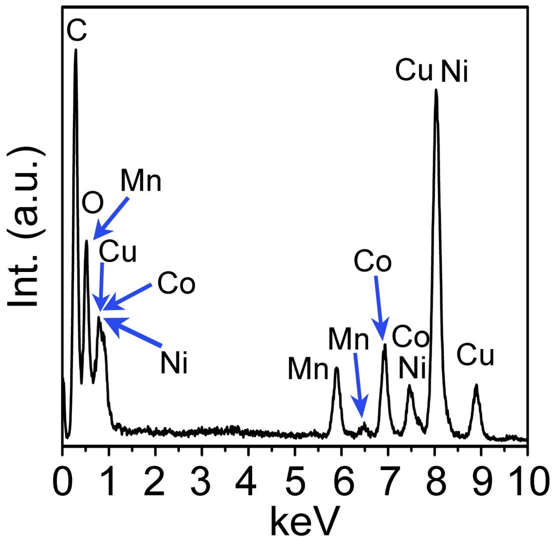
Figure S3. EDX spectrum of the hierarchical mesoporous  $\text{NiCo}_2\text{O}_4@\text{MnO}_2$  core-shell nanowires.
