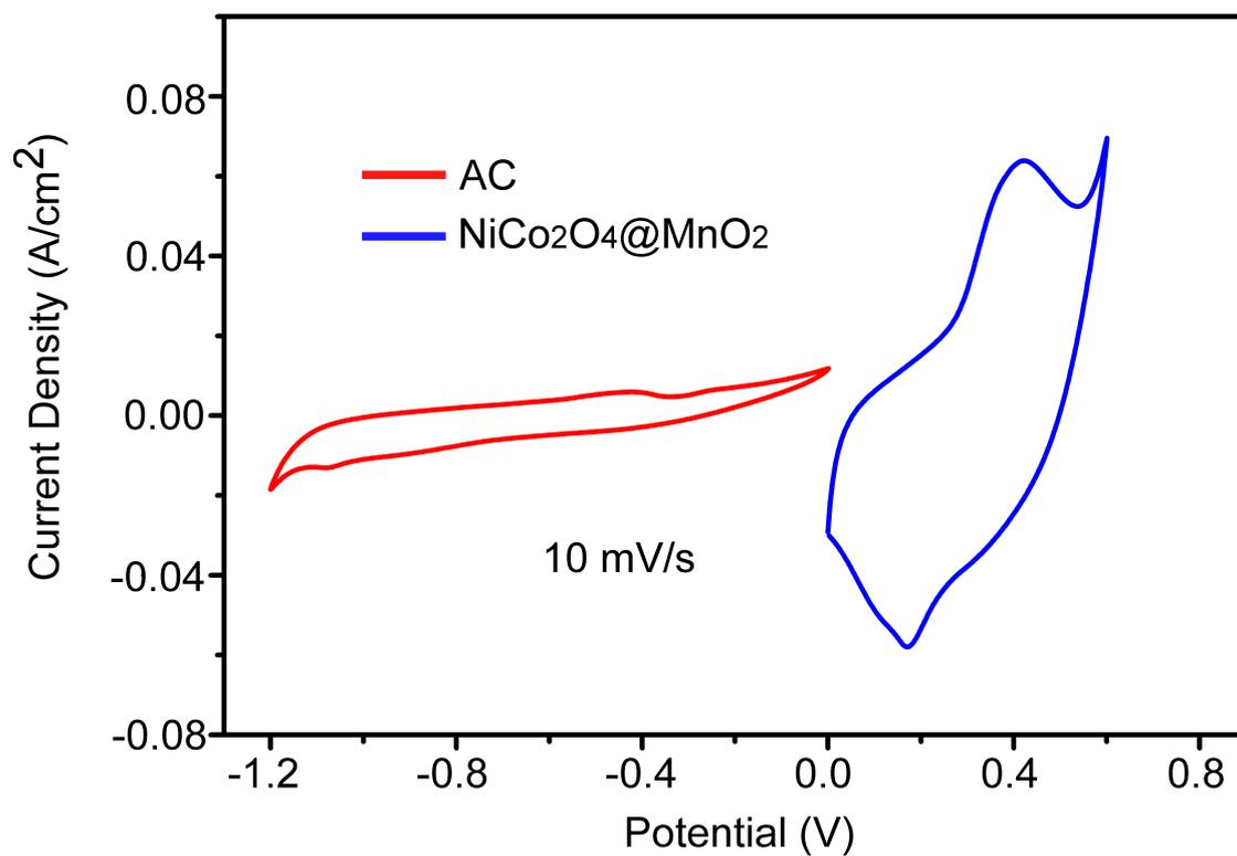
Figure S10. Comparative CV curves of the NiCo<sub>2</sub>O<sub>4</sub>@MnO<sub>2</sub> and activated carbon (AC) electrodes performed in a three-electrode cell at 10 mV/s.
