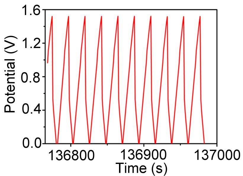
Figure S11. The CD curves of the last 10 cycles for the asymmetric supercapacitor.
