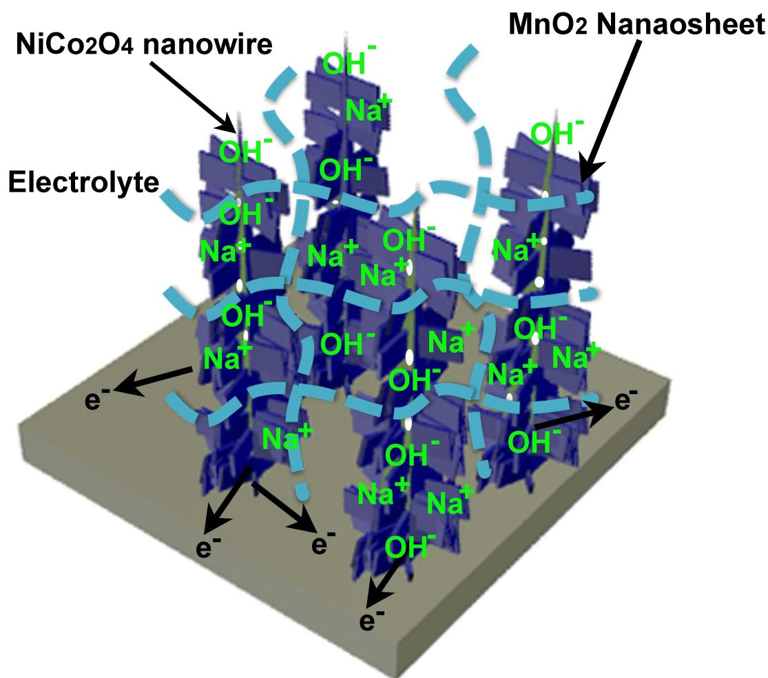
Figure S9. Schematic of the charge storage advantage of the hierarchical mesoporous  $\text{NiCo}_2\text{O}_4@\text{MnO}_2$  core-shell nanowire arrays on Ni foam, in which both the  $\text{NiCo}_2\text{O}_4$  core and  $\text{MnO}_2$  shell materials contribute to the charge storage.
