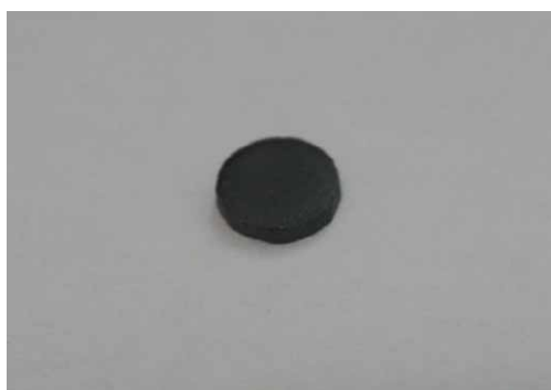
Figure S6. A photograph showing La-doped SrTiO 3 nanostructured bulk pellet (9.0% La) prepared by SPS.
