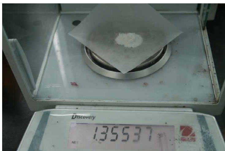
Figure S5. A photograph showing 1.35g of La-doped SrTiO 3 nanoparticles treated surfactant-removal process.
