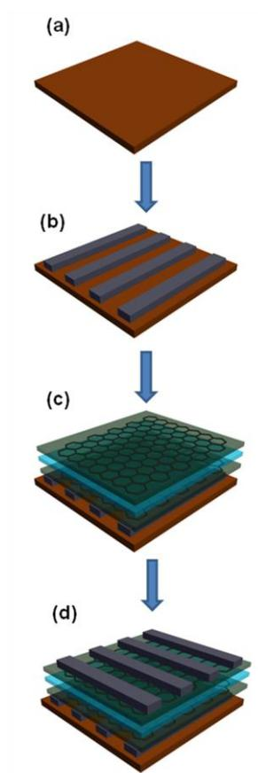
**Fig. S1.** Schematic diagram of fabrication process for dry conducting polymer actuator: (a) polyimide film, (b) deposition of bottom Al electrode, (c) spin coating of trilayer actuator configuration (active layer/solid polymer electrolyte/active layer), and (d) deposition of top Al electrode.
