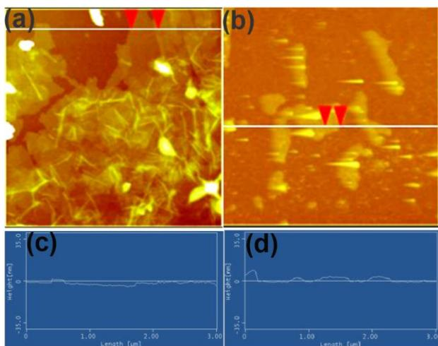
**Fig. S5.** Atomic force microscopy images of (a) GO and (b) GO-f-PTAA-co-PTh composites.
