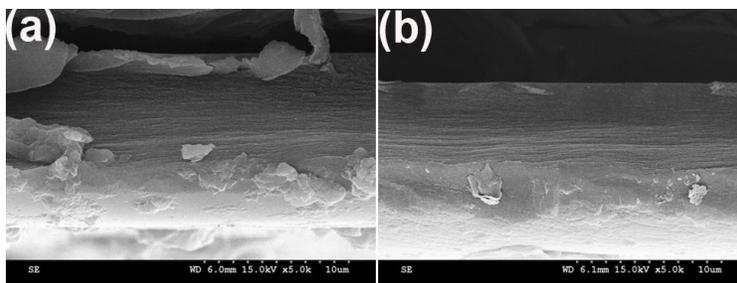
**Fig. S6.** Cross-sectional scanning electron microscopy images of GO-f-PTAA-co-PTh actuator device.
