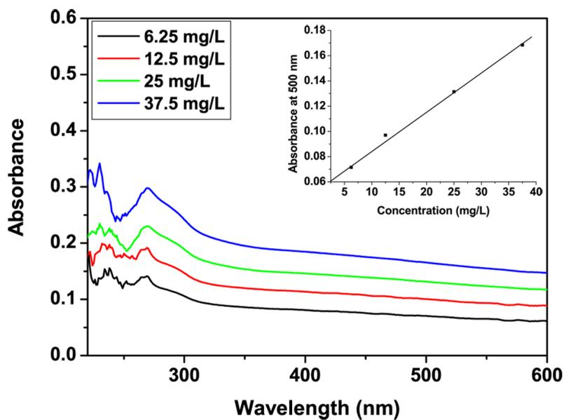
**Fig. S2.** Concentration dependence of UV-Vis absorption spectra of GO-f-PTAA-co-PTh in DMF solution with different concentrations of 6.25, 12.5, 25, and 37.5 mg/L. The inset shows the absorbance at 500 nm of the solution with different concentration.
