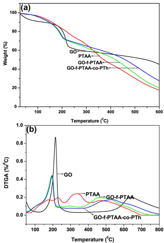
**Fig. S4.** (a) Thermogravimetric (TGA) curves of GO, PTAA, GO-f-PTAA, and GO-f-PTAA-co-PTh composites and (b) derivative TGA curves of the respective samples.
