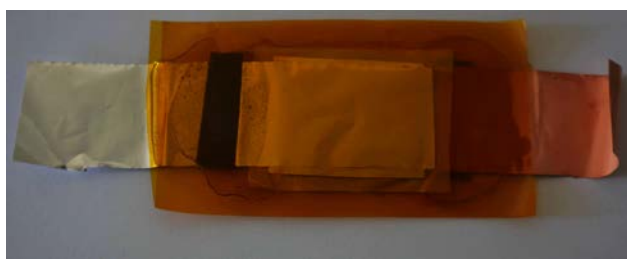
Figure S5. Photograph of a flexible full battery based on MoS 2 nanoflake arrays/carbon cloth-liquid electrolyte-LiCoO 2 full battery.
