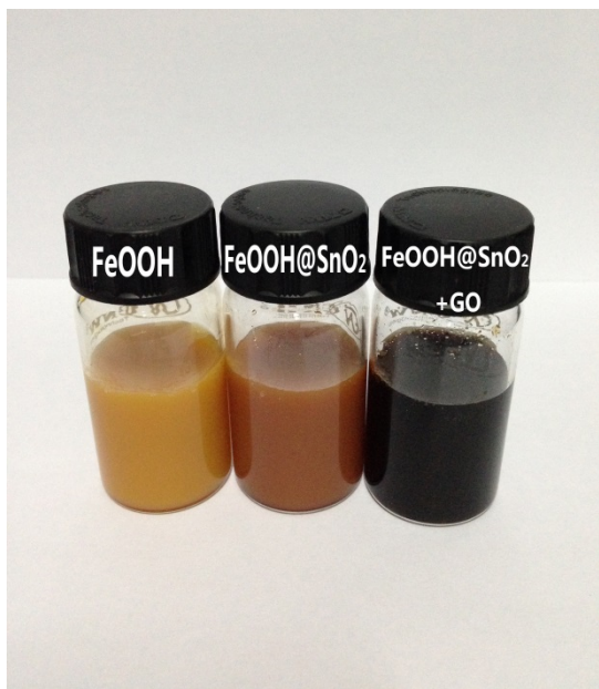
Fig. S2 Images of water dispersion of FeOOH nanoparticles (left) and FeOOH@SnO 2 nanoparticles (middle), dispersion of FeOOH@SnO 2 nanoparticles in GO water solution (right).
