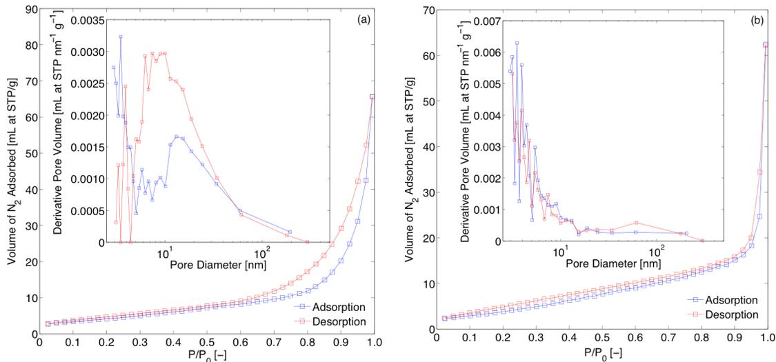
**Figure S1.**  $\text{N}_2$  physisorption isotherms (measured at  $-196^\circ\text{C}$ ) and pore size distributions (insets) of (a)  $\text{meso-Ca}_x\text{Al}_y\text{O}_z$  and (b)  $\text{CaO/meso-Ca}_x\text{Al}_y\text{O}_z$ .
