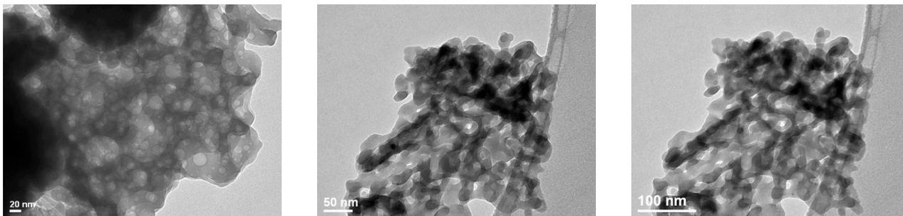
**Figure S2.** Transmission electron microscope images of  $\text{meso-Ca}_x\text{Al}_y\text{O}_z$ .
