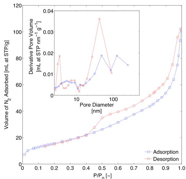
**Figure S12.**  $N_2$  physisorption isotherm (measured at  $-196\text{ }^\circ\text{C}$ ) and pore size distribution (inset) of  $\text{CaO}/\text{meso-Ca}_x\text{Al}_y\text{O}_z(20)$ .
