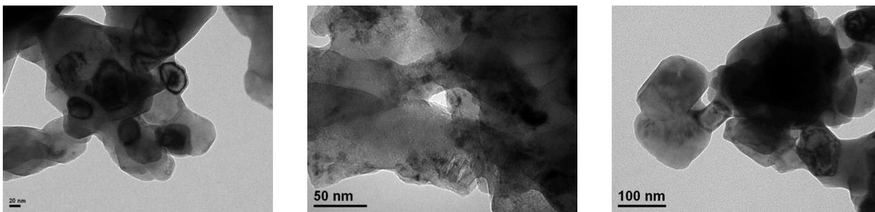
**Figure S3.** Transmission electron microscope images of  $\text{CaO/meso-Ca}_x\text{Al}_y\text{O}_z$ .
