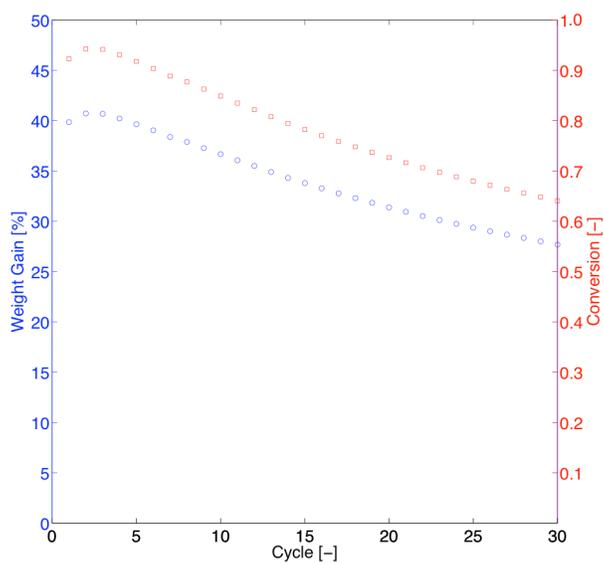
**Figure S14.** Performance of  $\text{CaO}/\text{meso-Ca}_x\text{Al}_y\text{O}_z(20)$  in 30 calcination-carbonation cycles (carbonation:  $700\text{ }^\circ\text{C}$ , 15%  $\text{CO}_2$  in  $\text{N}_2$ , 30 min; calcination:  $850\text{ }^\circ\text{C}$ ,  $\text{N}_2$ , 10 min).
