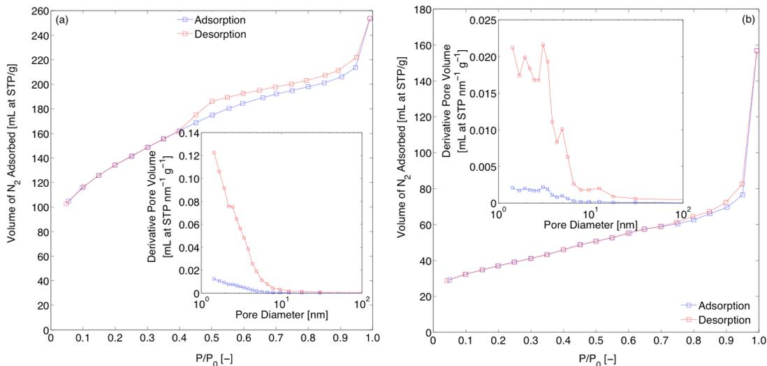
**Figure S7.** N<sub>2</sub> physisorption isotherms (measured at -196 °C) and pore size distributions (insets) of (a) *meso*-SiC and (b) CaO/*meso*-SiC.
