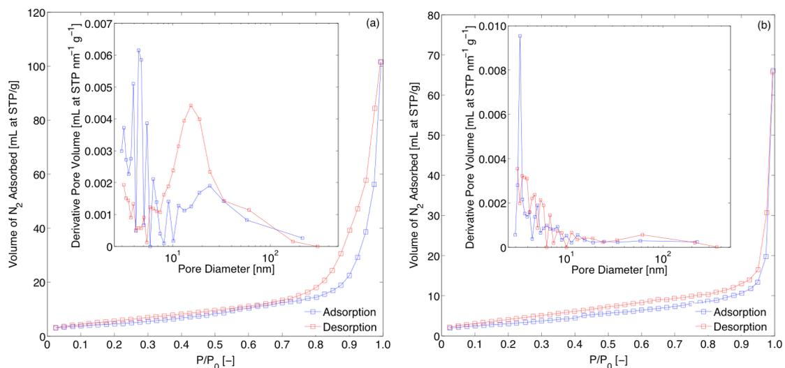
**Figure S4.**  $N_2$  physisorption isotherms (measured at  $-196^\circ C$ ) and pore size distributions (insets) of (a) *hier-Ca<sub>x</sub>Al<sub>z</sub>O<sub>z</sub>* and (b) *CaO/hier-Ca<sub>x</sub>Al<sub>z</sub>O<sub>z</sub>*.
