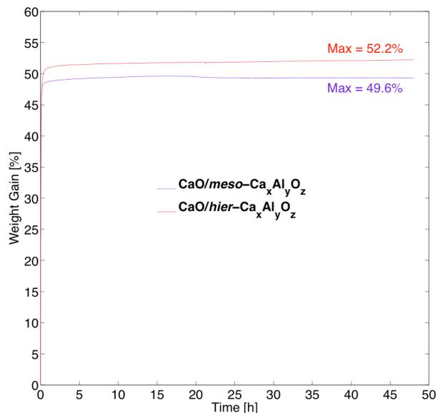
**Figure S11.** Determination of maximum carbonation levels for calcium aluminate sorbents. Samples were heated to 700 °C in 100%  $\text{CO}_2$ .
