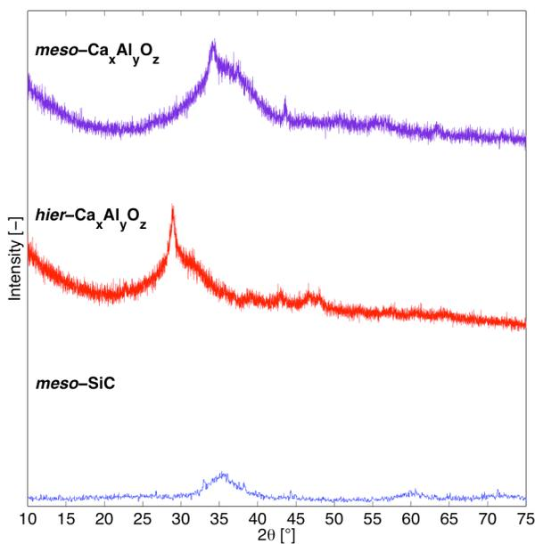
**Figure S10.** X-ray diffraction patterns of *meso-Ca<sub>x</sub>Al<sub>y</sub>O<sub>z</sub>*, *hier-Ca<sub>x</sub>Al<sub>y</sub>O<sub>z</sub>*, and *meso-SiC*. Each pattern was normalised and offset for plotting.
