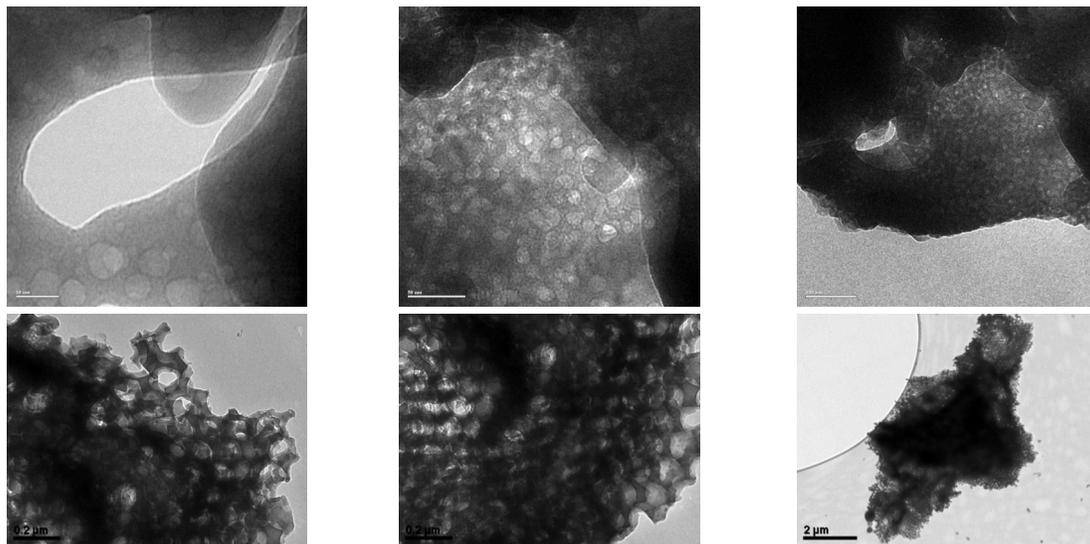
**Figure S5.** Transmission electron microscope images of *hier-Ca<sub>x</sub>Al<sub>z</sub>O<sub>z</sub>*.
