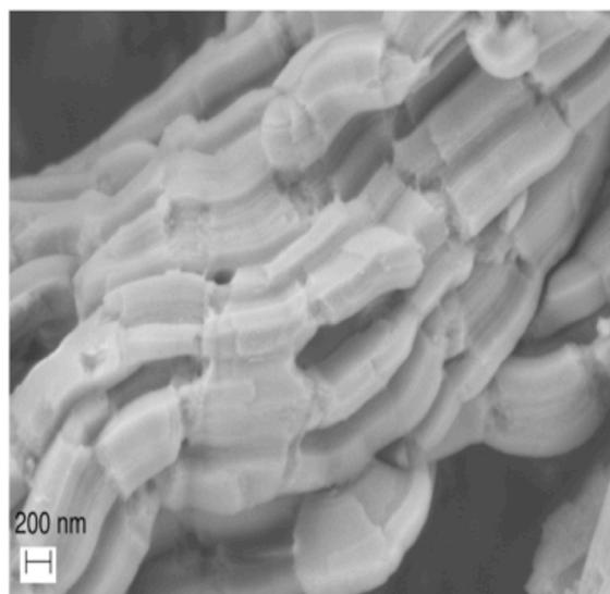
**Figure S8.** TEM (left) and SEM (right) images of SBA-15. TEM image of SBA-15, showing highly ordered mesoporosity. For TEM, the ultrafine sample that was obtained by sonicating the SBA-15 in ethanol was dispersed on a copper grid for measurement, and imaged using a 120-kV electron beam. For SEM, The sample was put on carbon tape and imaged using a secondary-electron detector and a 2-kV electron beam.
