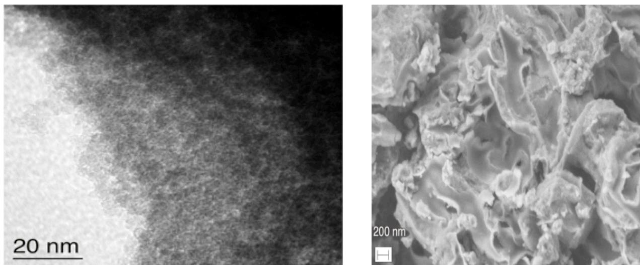
**Figure S9.** TEM (left) and SEM (right) images of *meso-SiC*. The ultrafine sample that was obtained by sonicating *meso-SiC* in ethanol was dispersed on a copper grid for measurement, and imaged using a 120-kV electron beam. For SEM, the sample was put on carbon tape and imaged using a secondary-electron detector and a 2-kV electron beam.
