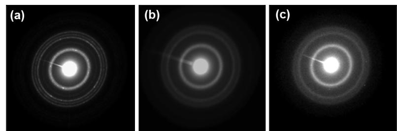
**Fig. S3** SAED patterns of the ZnS samples deposited at different IL-H<sub>2</sub>O interfaces: (a),  $[C_8\text{mim}][\text{PF}_6]\text{-H}_2\text{O}$ ; (b),  $[C_8\text{mim}][\text{Tf}_2\text{N}]\text{-H}_2\text{O}$ ; and (c),  $[C_8\text{mim}][\text{BF}_4]\text{-H}_2\text{O}$ .
