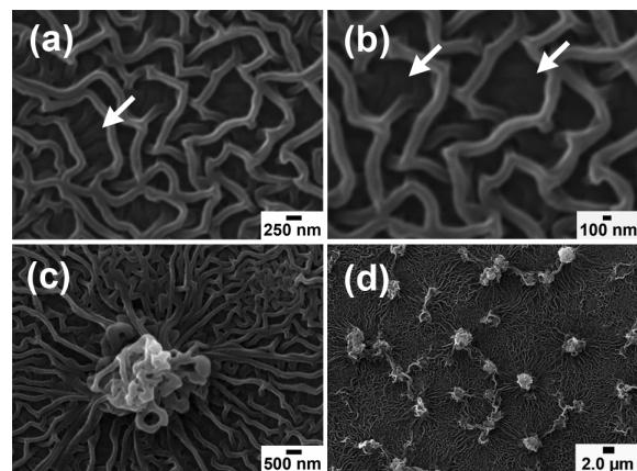
**Fig. S2** SEM images of the ZnS films prepared at 50 °C for 5 h of reaction at  $[C_8\text{mim}][\text{Tf}_2\text{N}]\text{-H}_2\text{O}$  interfaces: (a) and (b), high magnified dragon parts, and (c) and (d), different magnified flower parts.
