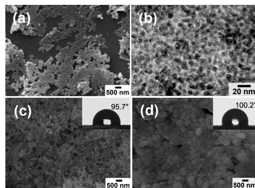
**Fig. S4** (a) SEM and (b) TEM images of the ZnS films prepared at 50 °C for 5 h of reaction at [C<sub>4</sub>mim][PF<sub>6</sub>]-H<sub>2</sub>O interface; (c), SEM image of the ZnS films prepared at 25 °C for 10 h of reaction at [C<sub>4</sub>mim][PF<sub>6</sub>]-H<sub>2</sub>O interface; and (d), SEM image of the ZnS films prepared at 60 °C for 5 h of reaction at [C<sub>4</sub>mim][PF<sub>6</sub>]-H<sub>2</sub>O interface.
