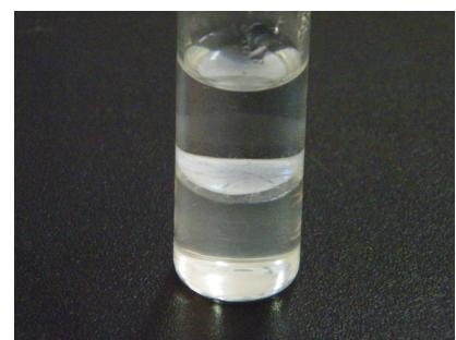
**Fig. S1** Photo of ZnS film deposited at the interface of  $[C_4\text{mim}][\text{PF}_6]\text{-H}_2\text{O}$  at 50 °C for 5 h of reaction.
