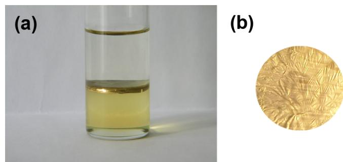
**Fig. S9** Photos of gold films deposited at the interface of [C<sub>8</sub>mim][Tf<sub>2</sub>N]-H<sub>2</sub>O (the pale yellow of subphase is the color of IL): (a), side view; and (b), top view.
