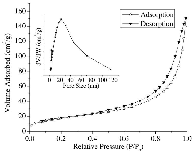
Figure S1.  $\text{N}_2$  adsorption-desorption isotherm and pore size distribution curve of RMMCMs
