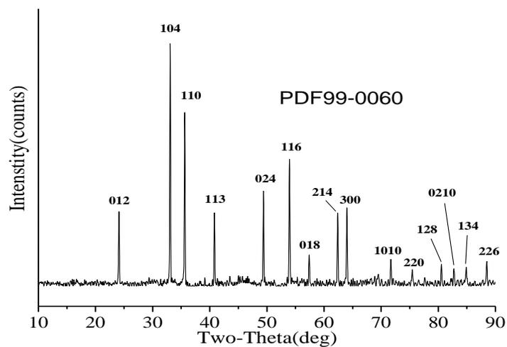
Figure S3 the XRD patterns of the  $\text{Fe}_2\text{O}_3$  powder obtained under  $200^\circ\text{C}$ , 4h without adding *Chlorella pyrenoidosa*.
