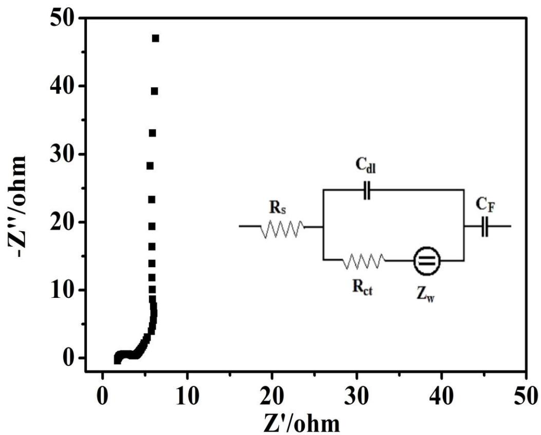
**Fig. S3** Nyquist plot of the NiO/GF//HPNCNTs asymmetric supercapacitor with the equivalent circuit in the inset.
