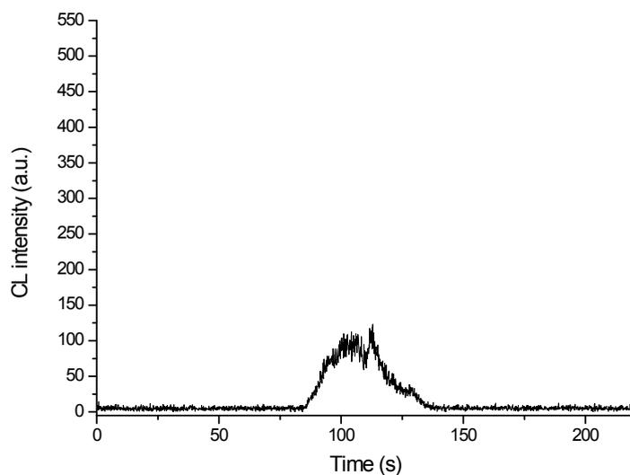
Figure S4 Response curves of H<sub>2</sub>S on VAFe/GN paper at 130°C. The detection limit of the as-prepared VAFe/GN is about 9ppm H<sub>2</sub>S at 130°C. The air flow rate is 200 ml/min.
