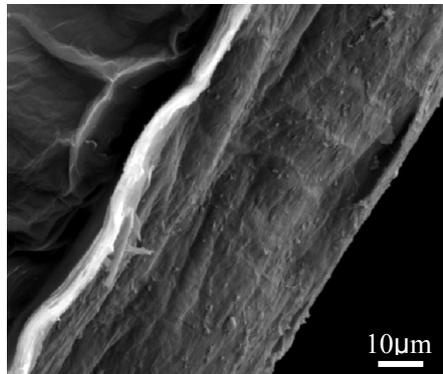
Figure S5. Cross section SEM image of HAFe/GN.
