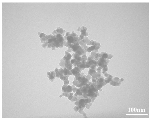
Figure S1. TEM image of aggregated Fe<sub>2</sub>O<sub>3</sub> nanoparticles synthesized in the absence of graphene.
