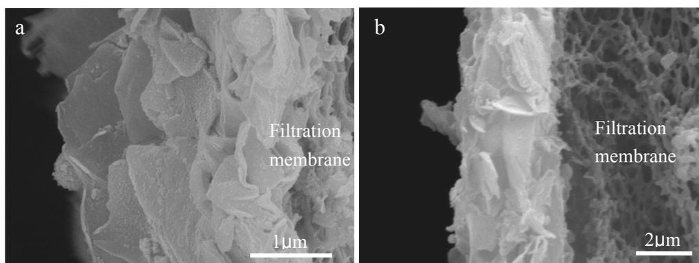
Figure S3. VAFe/GN films with different thickness. (a)  $\sim 2\mu\text{m}$  thick, (b)  $\sim 4\mu\text{m}$  thick.
