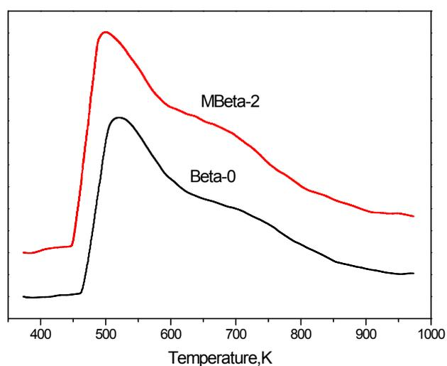
NH<sub>3</sub>-TPD of the samples was carried out in a flow-type fixedbed reactor. Firstly, the sample was exposed to flowing 5% NH<sub>3</sub>/He gas for a long time, and then purged by He at 423K to remove excessive physisorbed ammonia. The NH<sub>3</sub> desorption was conducted between 423 and 973K at a heating rate of 10K /min.
