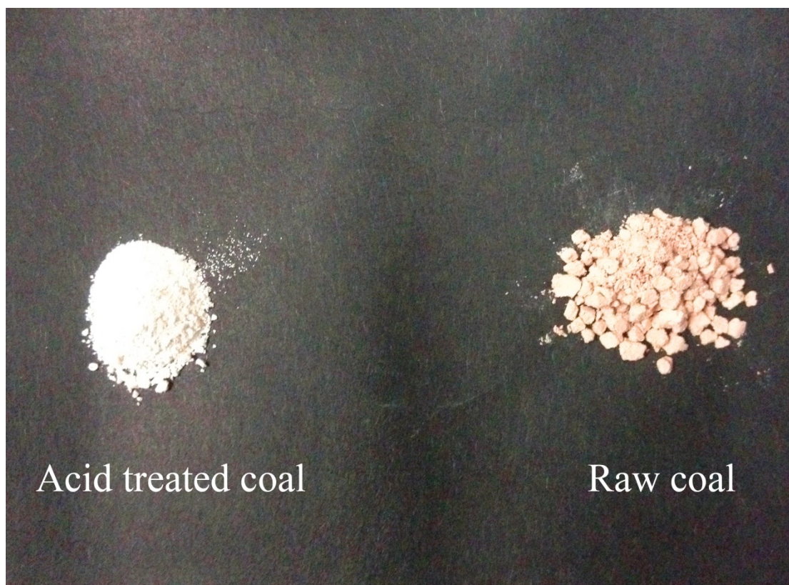
Fig S1 Optic photograph of ash of acid treated coal and raw coal
