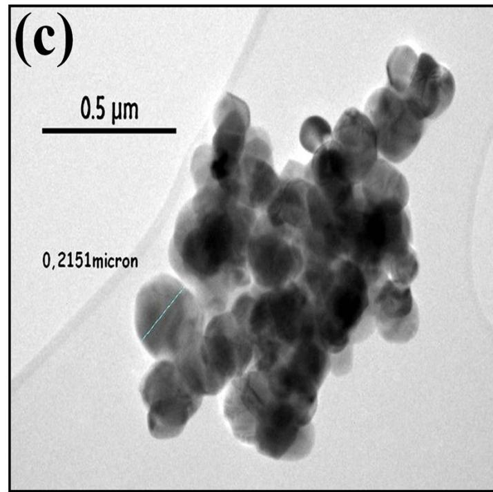
**Fig. S11** TEM images of (a) 3-5 nm sized  $\text{TiO}_2$  nanoparticles (b) 21 nm sized  $\text{TiO}_2$  nanoparticles and (c) bulk  $\text{TiO}_2$  particles
