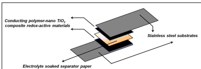
**Fig. S9** Schematic representation of the symmetric pseudo-capacitor device
