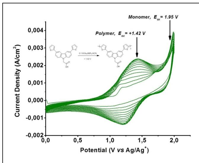
**Fig. S8** Cyclic voltammogram of TCAA in  $0.1 \text{ M} \text{ Bu}_4\text{NPF}_6/\text{ACN}$  at a scan rate of  $150 \text{ mV s}^{-1}$
