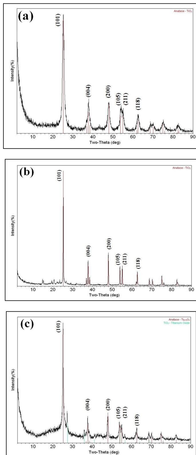
**Fig. S12** XRD patterns of the heterostructured (a) pTCAA/TiO<sub>2</sub> (3-5 nm sized) (b) pTCAA/TiO<sub>2</sub> (21 nm sized) (c) pTCAA/TiO<sub>2</sub> (bulk)
