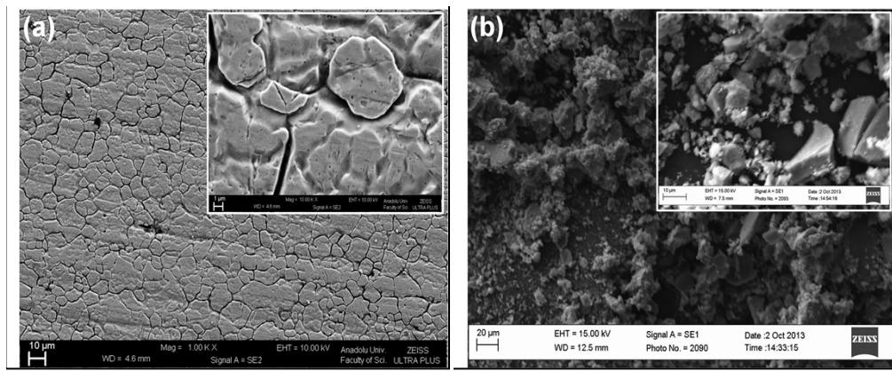
**Fig. S10** SEM images of (a) raw stainless steel substrate (b) 3-5 nm sized TiO<sub>2</sub> nanoparticles
