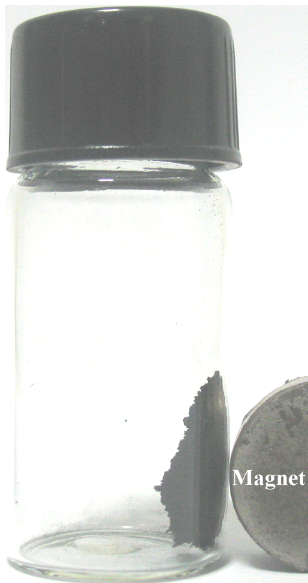
Fig. S3 Photograph showing the core/shell Co@C-60 attracted by a magnet after being soaked in 12 M HCl solution for four weeks.
