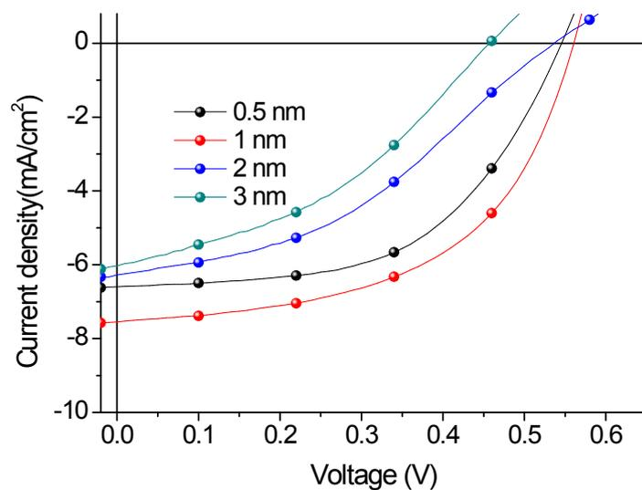
**Fig. S5** J-V curve for the inverted OPV with LiF at thicknesses varying from 0.5 nm to 3nm
