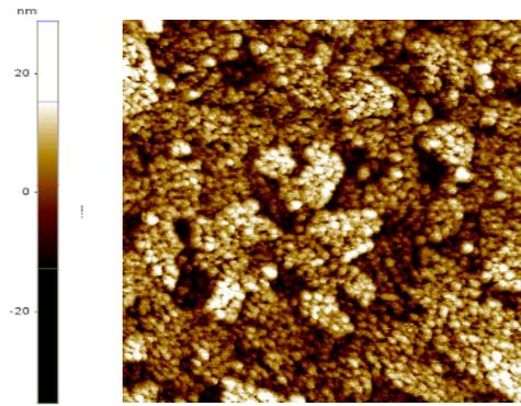
**Fig.S6** (a) AFM image of Yb (2 nm) on ITO (b) AFM image of LiF (2 nm) on ITO
