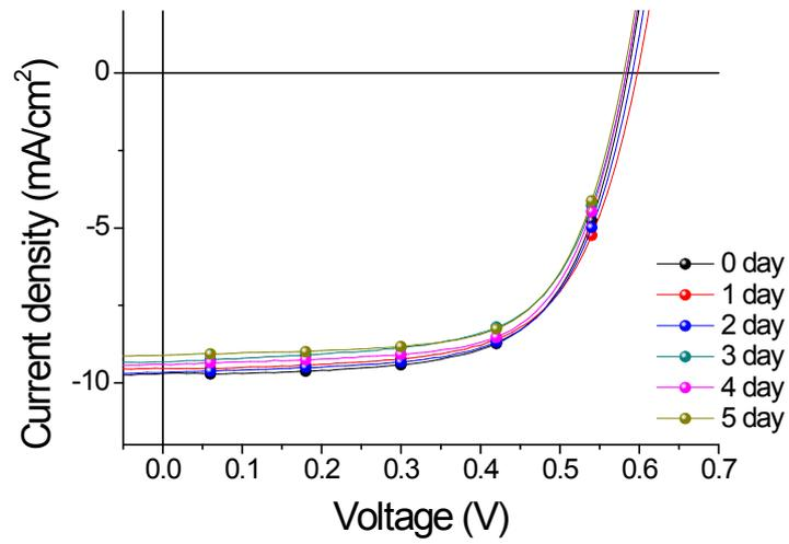
**Fig. S7** The J-V curve for the inverted OPV with PEIE over time.
