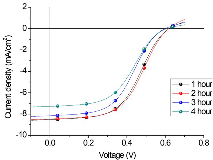
**Fig. S8** J-V curve of the OPV with Yb where Yb is exposed to ambient air before the deposition of the active layer under various exposure times
