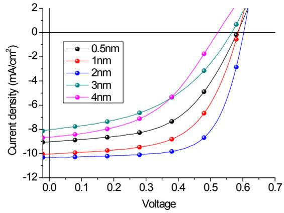
**Fig. S3** J-V curve of the inverted OPV featuring Yb with varying thicknesses
