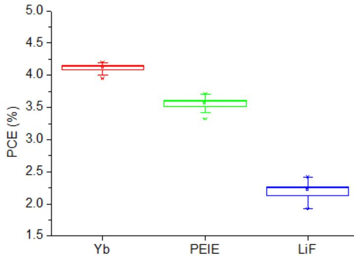
**Fig. S9** Box and whisker plot of the PCE of the inverted OPVs with each ETL.
