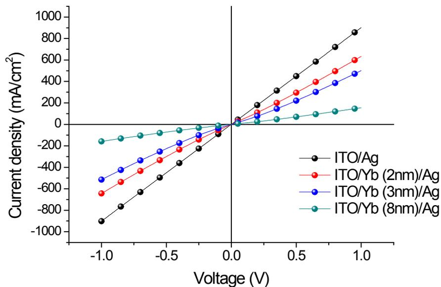
**Fig. S2** I-V curve for the samples composed of ITO/Yb(20 Å)/Ag and the samples composed of ITO/Ag
