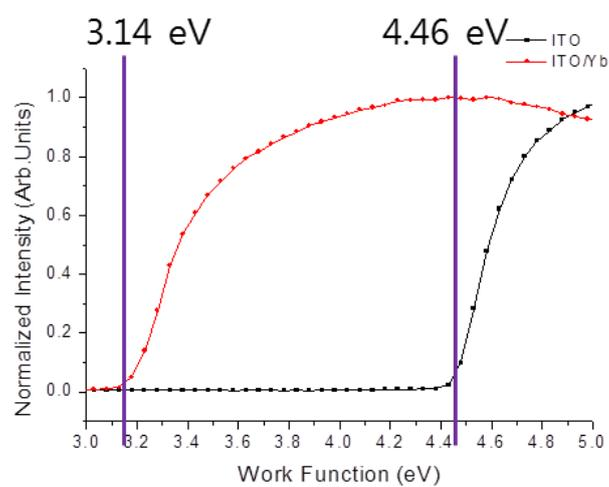
**Fig. S1** The work function of Yb on ITO and ITO by UPS analysis
