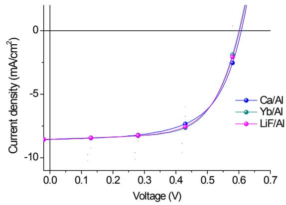
**Fig. S4** The J-V curve for the conventional OPVs with Ca, Yb and LiF as ETLs
