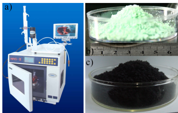
Figure S1. (a) Optical photographs of microwave reactor; (b), (c) the large-scale products of nickel hydroxide precursors (1.48 g) and NiO nanosheets (1.14 g) synthesized one times.
