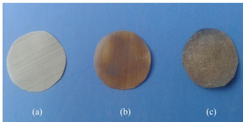
**Figure S1.** Photography of the SSN wafer (a), PDA-functionalized SSN wafer (b), and ZIF-8 membrane supported on PDA-functionalized SSN wafer (c).
