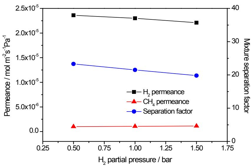
**Figure S4.** H<sub>2</sub>/CH<sub>4</sub> selectivity and permeances of the ZIF-8 membrane prepared on PDA-functionalized SSN as function of the H<sub>2</sub> partial pressure at 100 °C.
