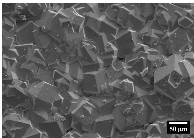
**Figure S2.** FESEM image of the ZIF-8 membrane layer prepared on PDA-functionalized SSN after 10 minutes ultrasonic treatment.
