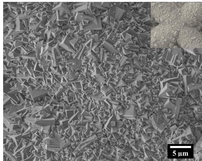
**Figure S3.** Top view FESEM image of the zeolite LTA membrane supported on PDA-functionalized SSN prepared at 60 °C for 24 h.
