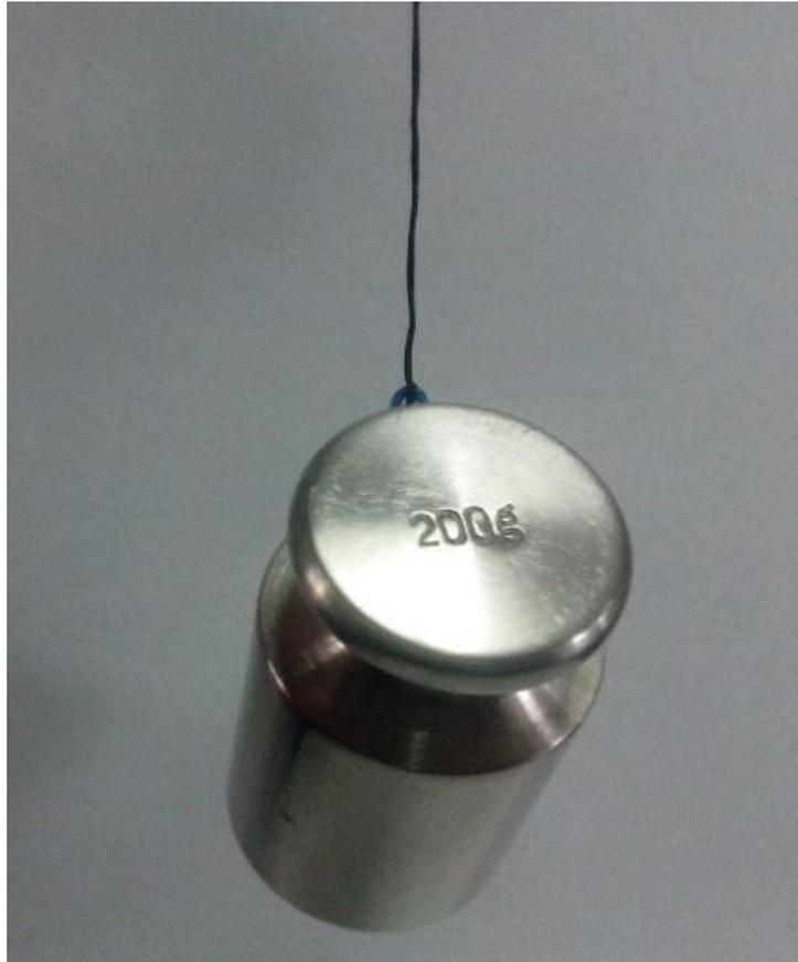
Figure S12. Images of a single GF which lift up a 200 g load.
