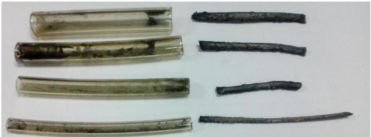
Figure S2. Photograph of the freeze-dried as-prepared wet-form GFs with different diameter released from the pipelines with the different inner diameter (from 2.5 to 8mm).
