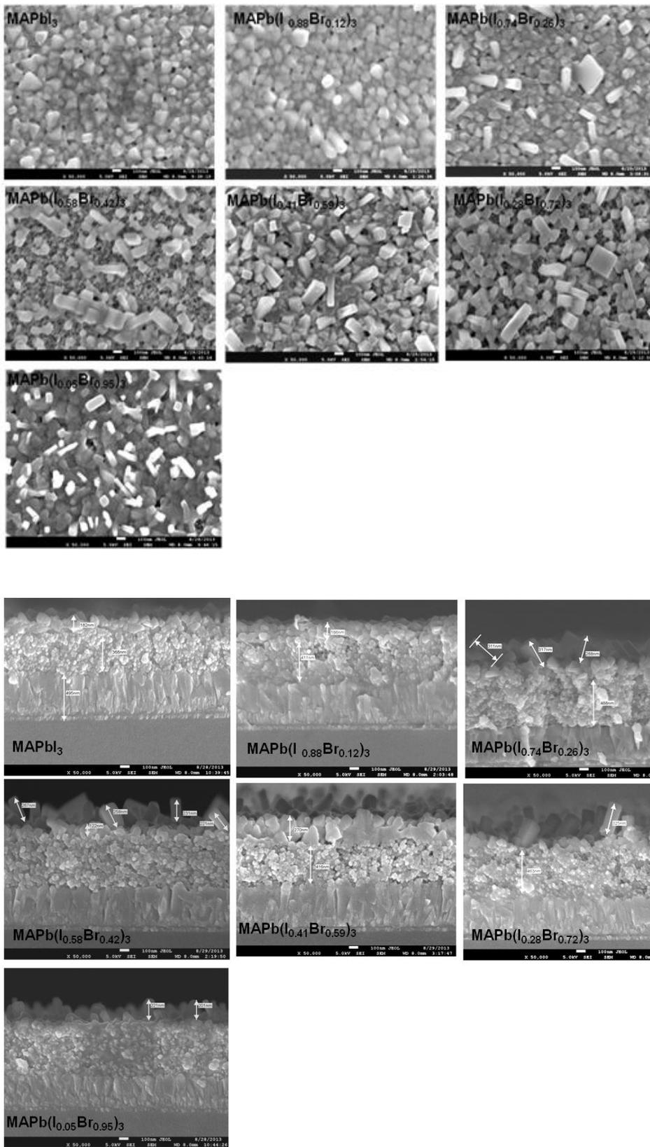
**Fig. S4:** Field emission microscopic (FESEM) images of the mixed halide perovskite films with different halide mixtures top & cross sectional view.
