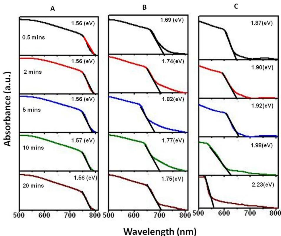
**Fig. S1:** Ex-situ UV-vis spectra of perovskite films formed by dipping PbI<sub>2</sub> films (on mp-TiO<sub>2</sub>/bl-TiO<sub>2</sub>/FTO substrate) at different time interval in: A) Methyl ammonium iodide (MAI), B) Mixture of Methyl ammonium iodide (MAI) & Methyl ammonium bromide (MABr) (1:1), and) Methyl ammonium bromide (MABr) solutions in isopropanol (IPA).
