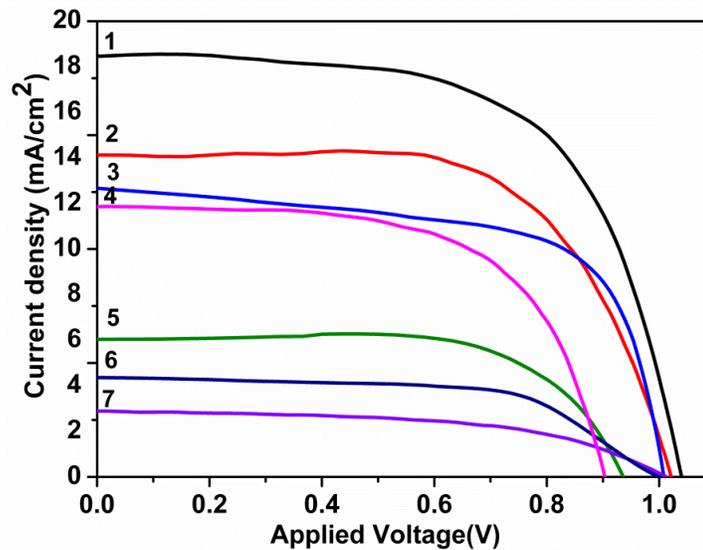
**Fig.S3** : The characteristic J-V curves of the mixed lead halide perovskite devices. The number 1 to 7 represents the composition of the mixed halide. 1.  $MAPbI_3$ , 2.  $MAPb(I_{0.88}Br_{0.12})_3$ , 3.  $MAPb(I_{0.74}Br_{0.26})_3$ , 4.  $MAPb(I_{0.58}Br_{0.42})_3$ , 5.  $MAPb(I_{0.41}Br_{0.59})_3$ , 6.  $MAPb(I_{0.28}Br_{0.72})_3$ , and 7.  $MAPb(I_{0.05}Br_{0.95})_3$ .
