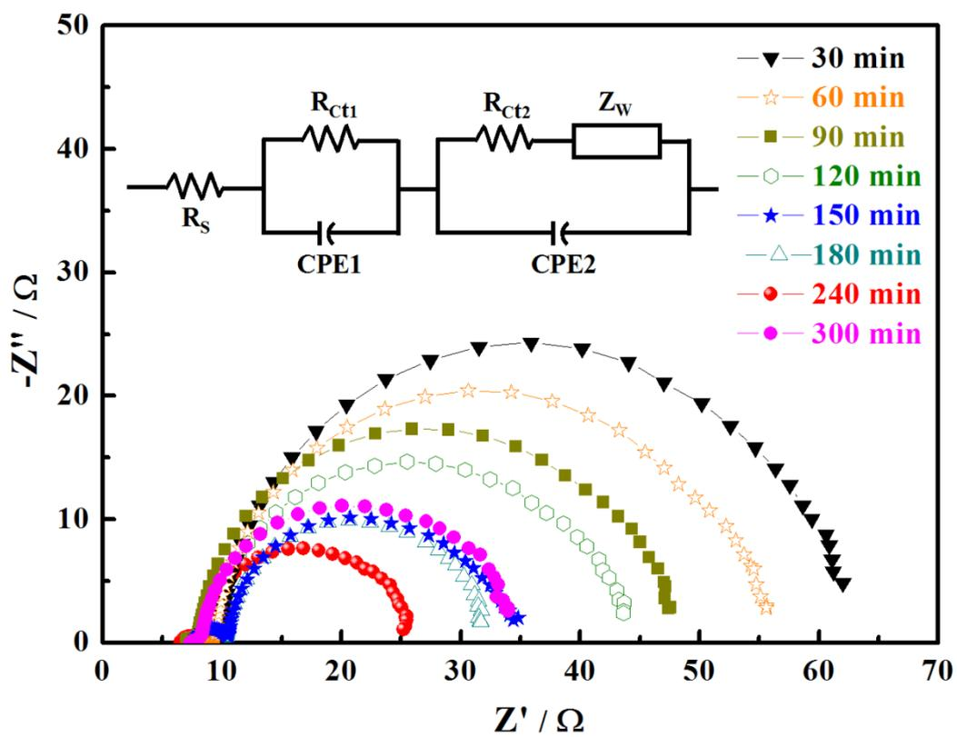
**Figure S5** EIS spectra of the DSSCs with TNT anodized at 50 V for 30, 60, 90, 120, 150, 180, 240, and 300 min, measured at  $100 \text{ mW cm}^{-2}$  under open-circuit voltage.
