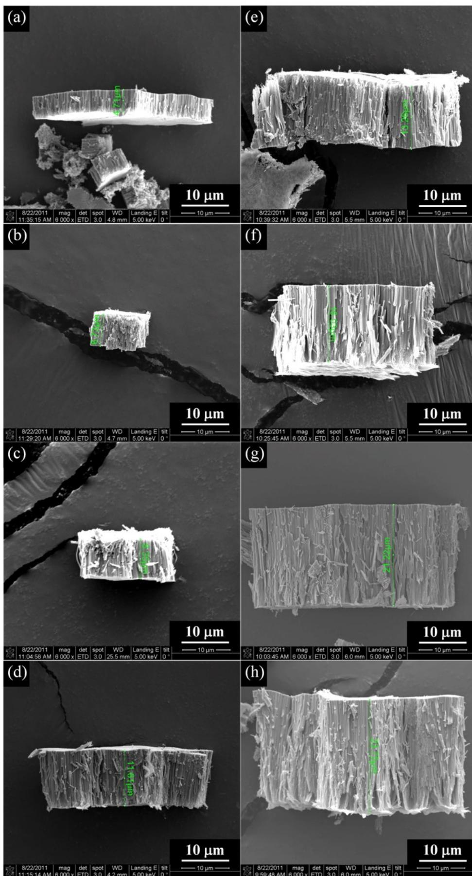
**Figure S3** SEM images of the side views of TNTs anodized at 50 V for (a) 30, (b) 60, (c) 90, (d) 120, (e) 150, (f) 180, (g) 240 and (h) 300 min.
