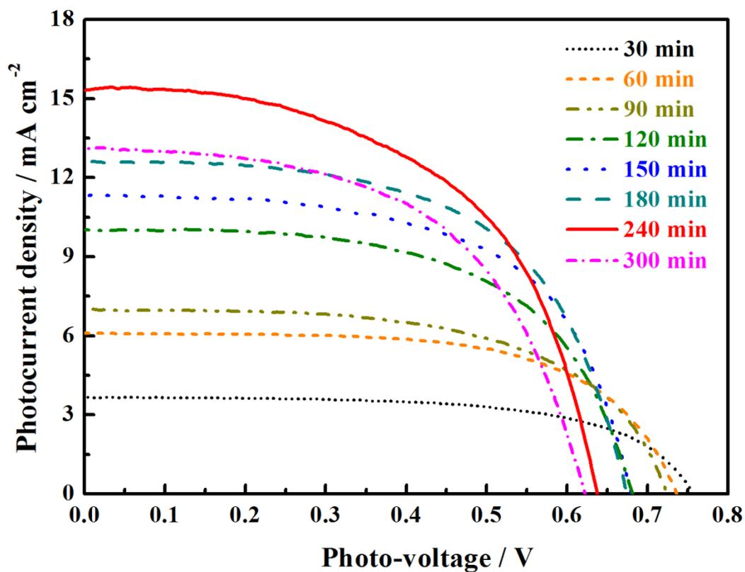
**Figure S4** Photocurrent density–voltage curves of the DSSCs with TNT anodized at 50 V for 30, 60, 90, 120, 150, 180, 240, and 300 min, measured at 100 mW cm<sup>-2</sup>.
