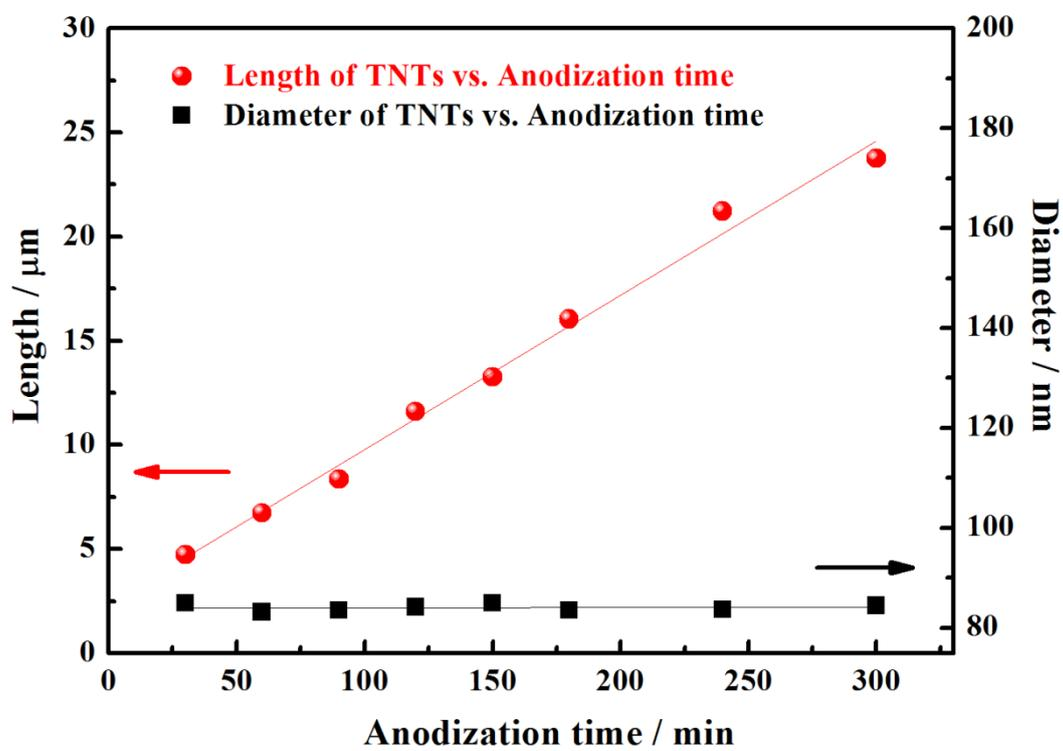
Figure S1 Dependence of the diameter and length of the TNT on the anodization period.
