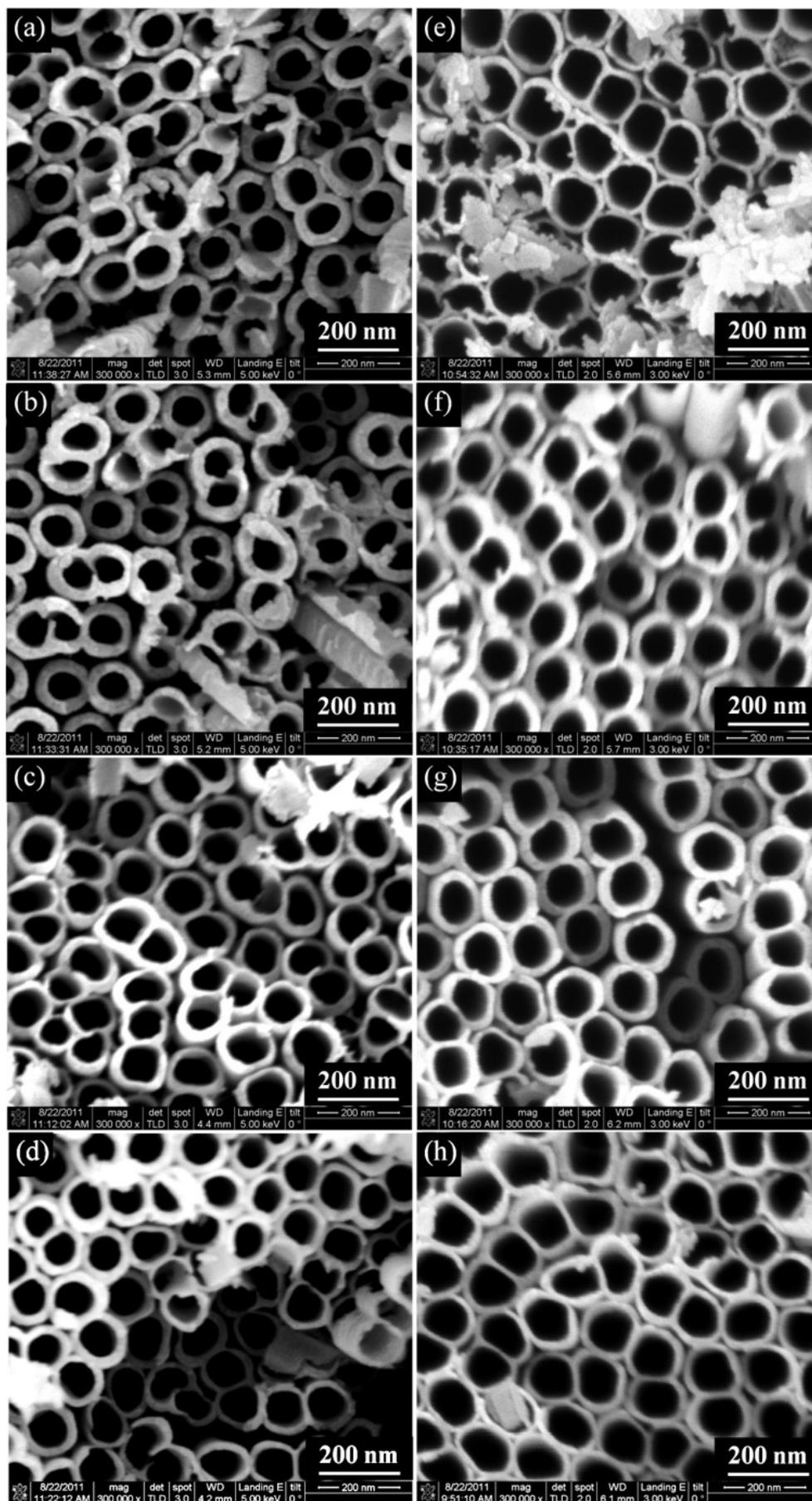
**Figure S2** SEM images of the top views of TNTs anodized at 50 V for (a) 30, (b) 60, (c) 90, (d) 120, (e) 150, (f) 180, (g) 240 and (h) 300 min.
