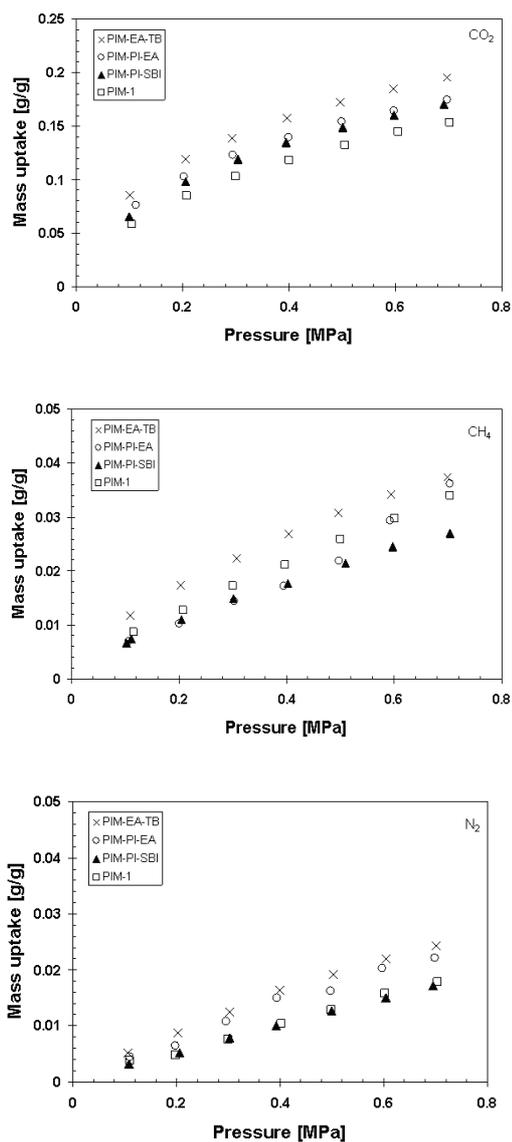
**ESI Figure 1.** Sorption isotherms for CO<sub>2</sub> (top), CH<sub>4</sub> (middle) and N<sub>2</sub> (bottom) in the four methanol treated polymers PIM-1, PIM-PI-SBI, PIM-EA-TB and PIM-PI-EA.
