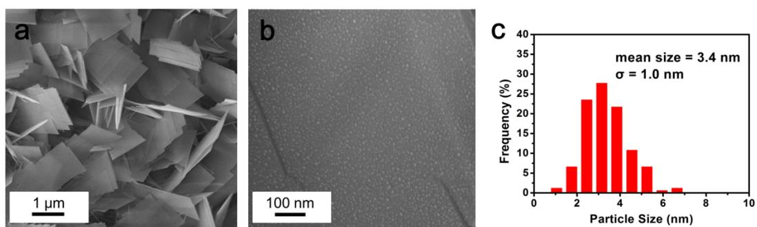
**Fig. S3** SEM images of 2.8 wt% Au/NiCoCH-NSAs (a, b) and corresponding particle size distribution histogram of Au loaded on NiCoCH-NSAs (c) after being recycle-used for six times.
