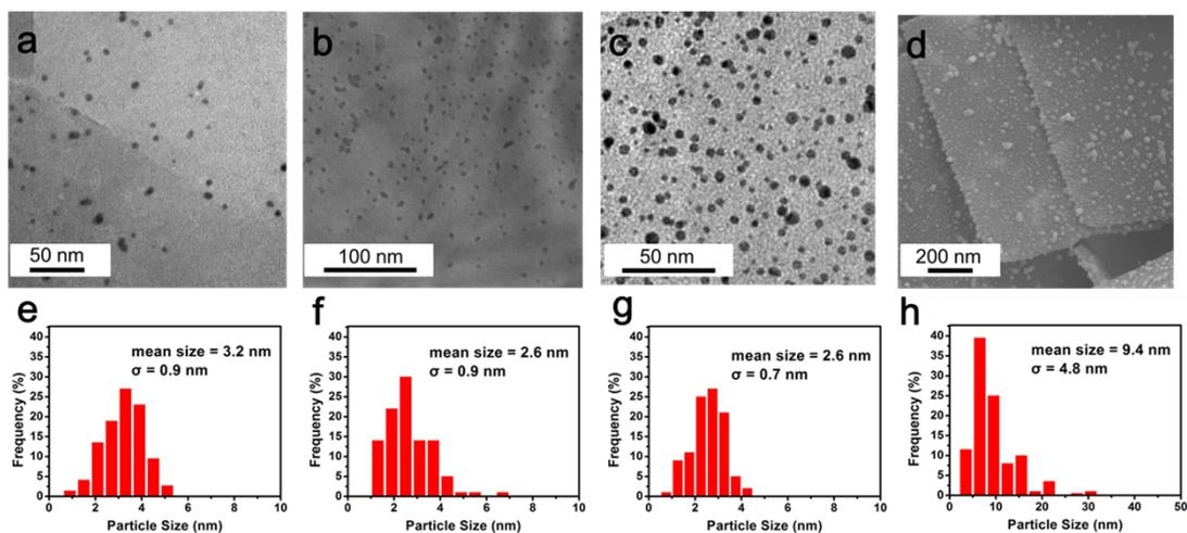
Fig. S2 TEM images of obtained (a) 0.1 wt%, (b) 0.7 wt% and (c) 2.8 wt% Au/NiCoCH-NSAs; (d) SEM image of obtained 8.1 wt% Au/NiCoCH-NSAs. (e-h) The corresponding Au particle size distribution histograms of Au/ NiCoCH-NSAs samples with different Au loading amount.
