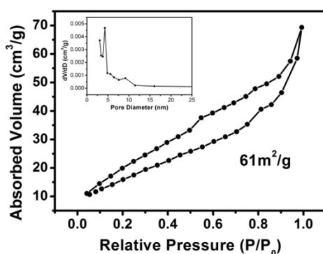
Fig. S1 N<sub>2</sub> adsorption–desorption isotherm and PSD (inset) of NiCoCH-NSAs.
