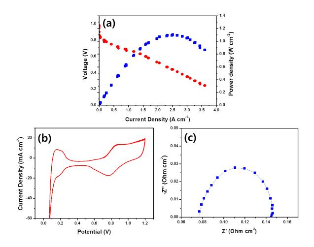
**Table S1**. Membrane properties and performance of of single PEM fuel cell MEAs fabricatedwith commercial Nafion 212 membrane at 75 °C 100 % RH.
