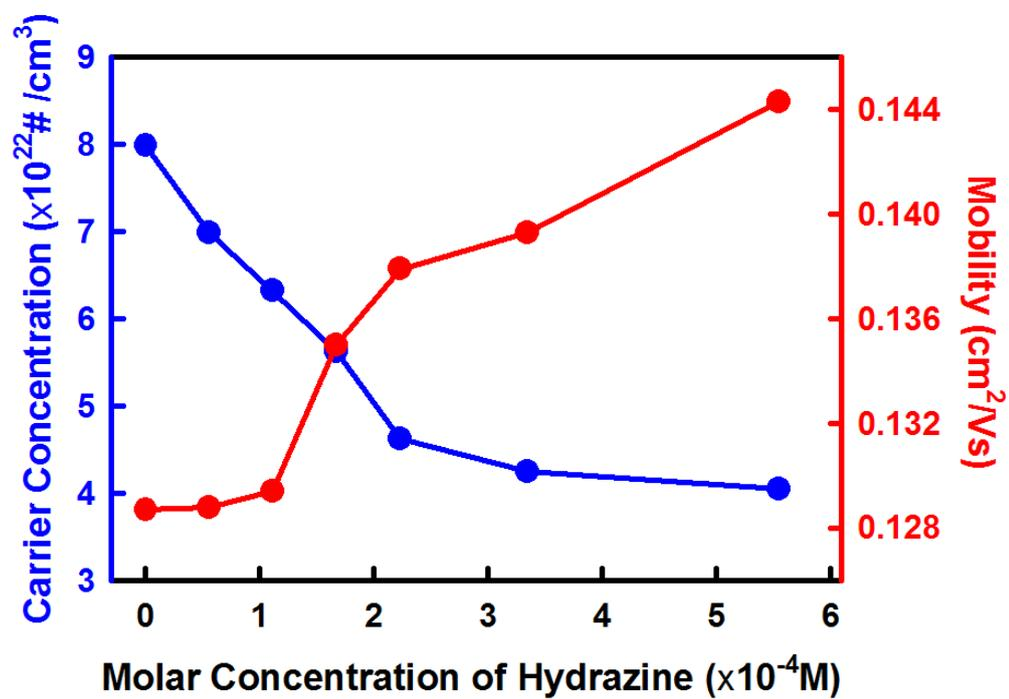
**Fig S1.** Variation of carrier concentration ( $n$ ) and mobility ( $\mu$ ) of hydrazine/DMSO-doped PEDOT:PSS (DDTP) films as a function of hydrazine concentration. The electrical conductivity ( $\sigma$ ) is proportional to  $n \times \mu$ .
