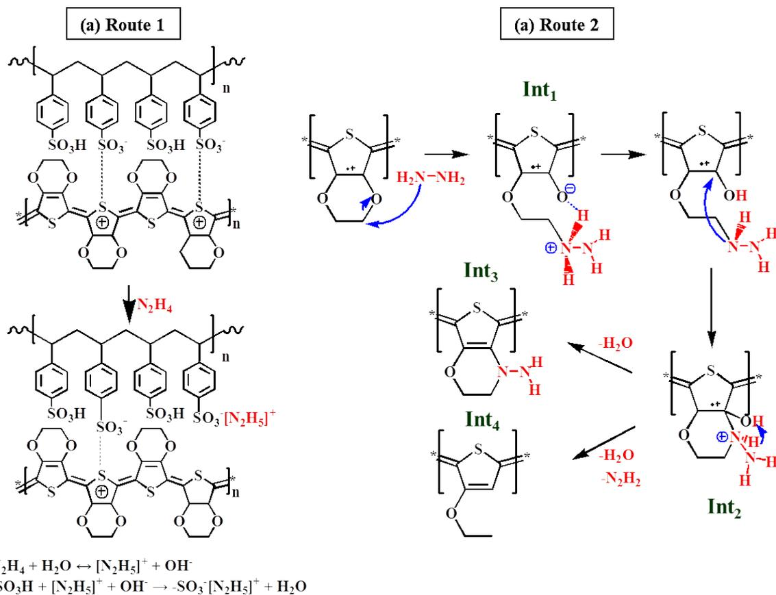
**Fig S2.** Dedoping and reduction mechanism of PEDOT:PSS films treated by hydrazine/DMSO (i.e. DDTP films): (a) dedoping of PEDOT:PSS film by the neutralization of PSS and (b) reduction of PEDOT molecules with excess amount of hydrazine as a reducing agent.
