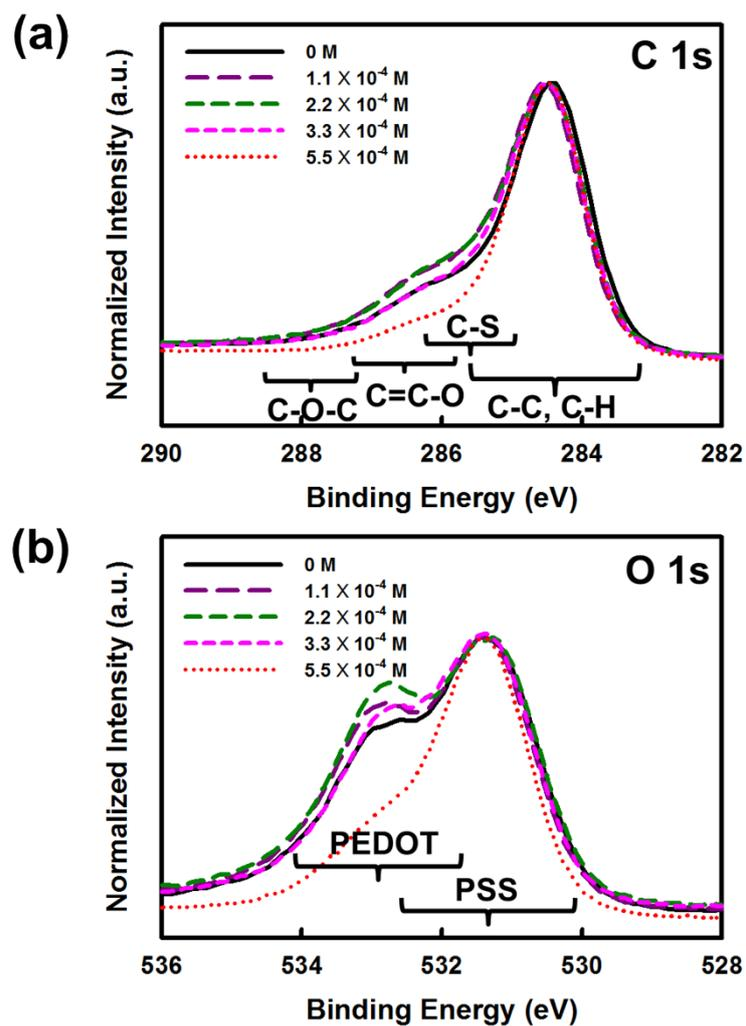
**Fig S3.** XPS spectra of the PEDOT:PSS films treated by hydrazine/DMSO with different hydrazine concentration (i.e. DDTP films): (a) C 1s and (b) O 1s XPS peaks.
