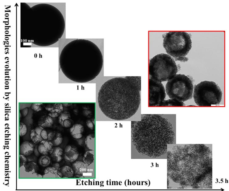
**Figure S1.** Morphologies evolution of  $\text{SiO}_2$  spheres during different etching times. The inset image with green frame indicates the unsuccessful templating from 2 hours etched samples, while the image labeled with red square indicates the successful templating from 3 hours etched samples.
