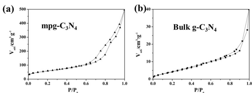
**Figure S4.**  $\text{N}_2$  sorption isotherms of mpg- $\text{C}_3\text{N}_4$  (a) and bulk g- $\text{C}_3\text{N}_4$ .
