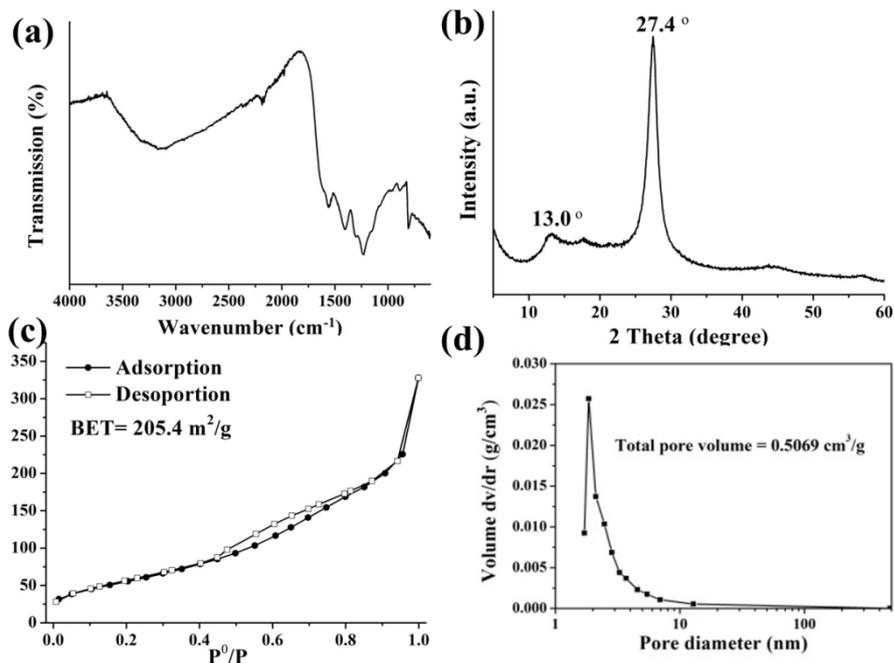
**Figure S3.** (a) FTIR spectrum of CNMS showing typical C-N heterocycle stretches in the 1100~1600  $\text{cm}^{-1}$  spectral range and the breathing mode of the tri-s-triazine units at 810  $\text{cm}^{-1}$ . (b) XRD spectrum of CNMS with two peaks at 13.0° and 27.4° ascribed to the in-planar repeat period and stacking of the conjugated aromatic system, respectively. (c)  $\text{N}_2$  sorption isotherm of CNMS with the pore size distribution plot in (d).
