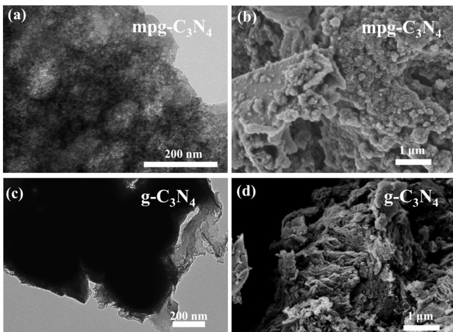
**Figure S5.** TEM and SEM characterizations of mpg- $C_3N_4$  (a and b) and g- $C_3N_4$  (c and d), respectively.
