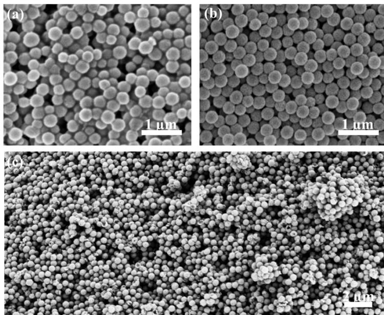
**Figure S2.** SEM images of silica before (a) and after etching (b). Image (c) illustrates the large area overview of CNMS.
