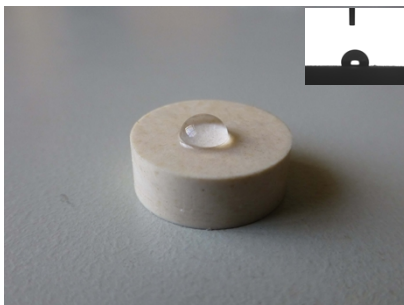
Fig. S4 A water droplet on the oil contaminated bulk material surface with water CA value about 120°.
